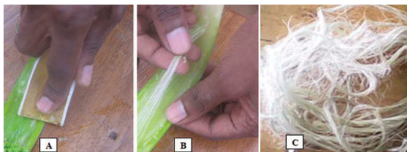
FIGURE 2 Manual extraction of STF: (A) hand scrutching; (B) lifting of STF; (C) extracted STF.
