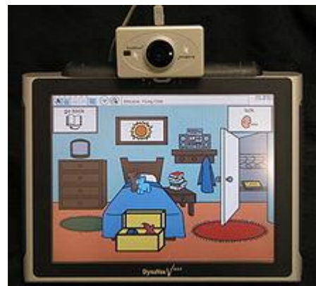
Speech generating device accessed using a head mouse
