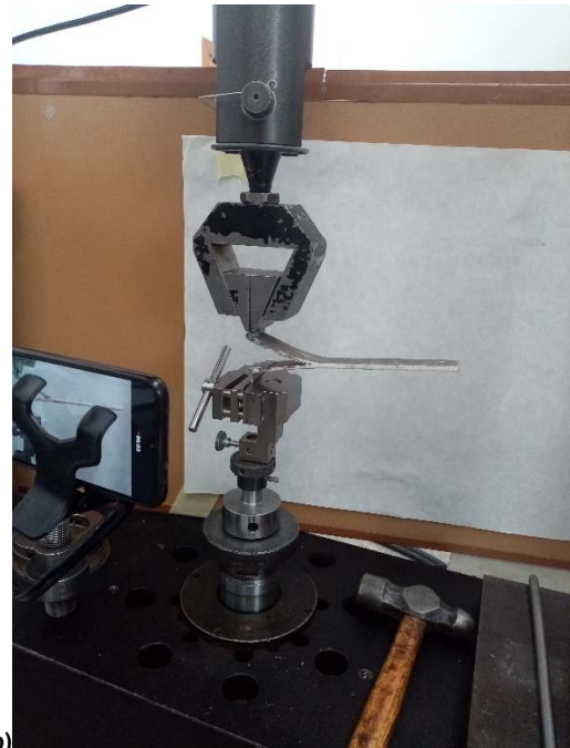
Figure 2a and 2b. 2a - Tensile strength and tensile elongation test; 2b - Interlaminar fracture toughness test [own source].
