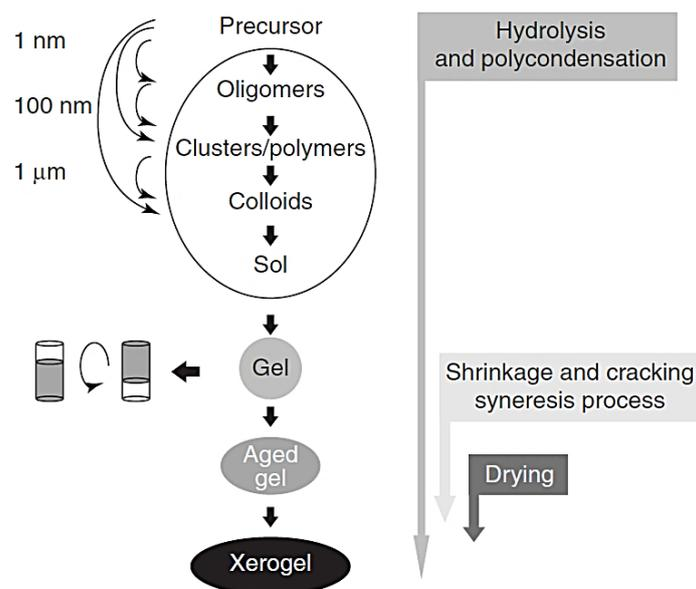
**Figure 5.** An overview of the transformations ongoing during the sol-gel process [43].
