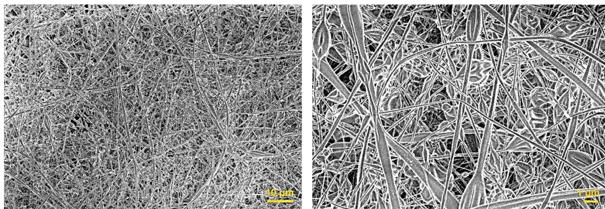
**Figure 52.** Disrupted hybrid organosilane fibers containing beads prepared from a combination of the BiTSAB precursor:TEOS 50 mol.% under different needle-electrospinning conditions.
