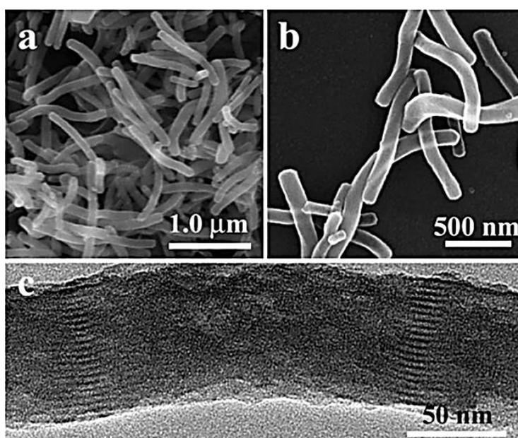
**Figure 24.** Electron microscopy images of the formation of mesoporous ethane-1,2-diyl – silica nanorods via the self-assembly process. FESEM microscopy **a)**; **b)** and TEM microscopy **c)** [133].
