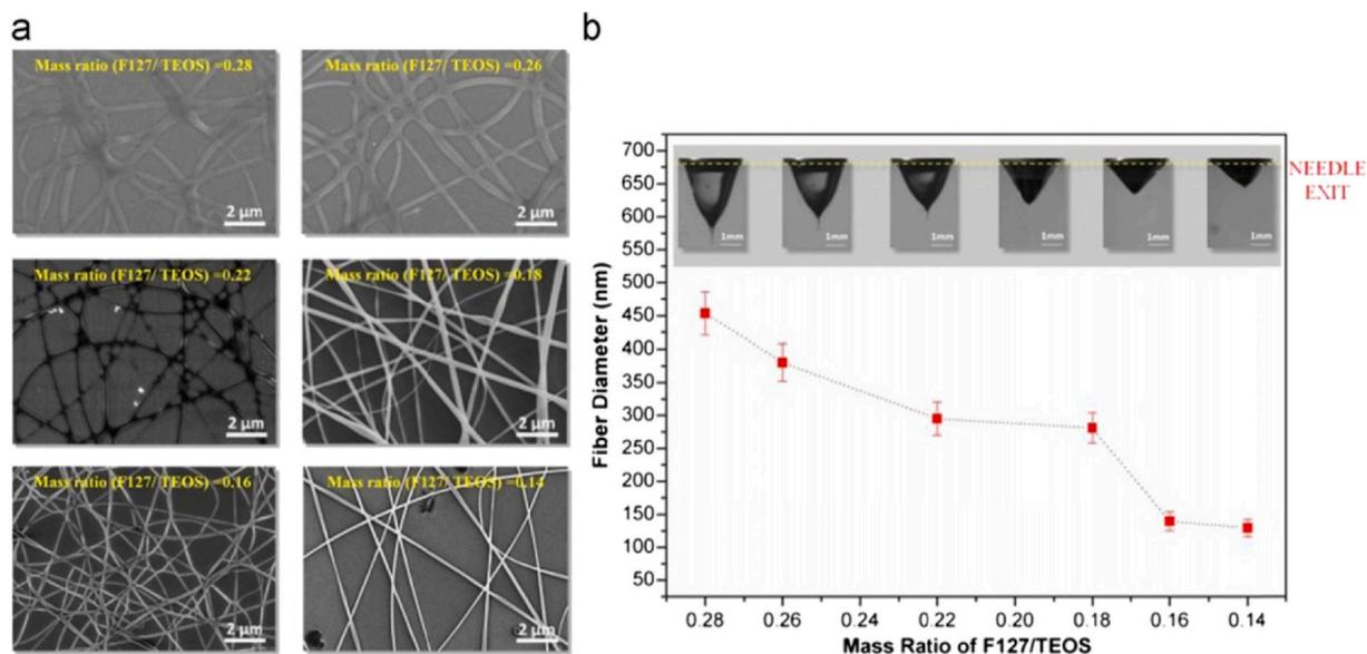
Fig. 11. SEM images of silica nanofibers prepared using sols with different F127/TEOS mass ratios a); and the relationship between the fiber diameter and the F127/TEOS mass ratios b); [107].
