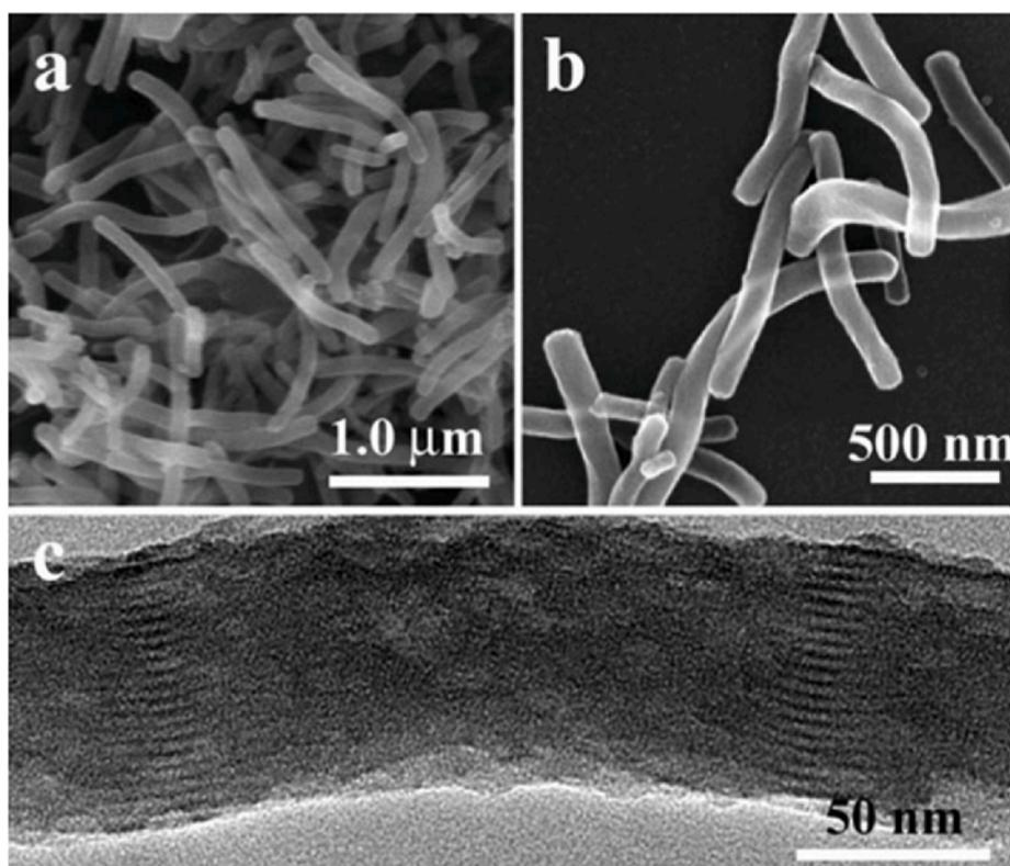
Fig. 15. Electron microscopy images of the formation of mesoporous ethane-1,2-diyl – silica nanorods via the self-assembly process. FESEM microscopy (a,b) and TEM microscopy (c) [116].
