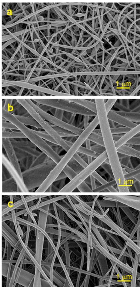
Fig. 4. SEM images of BIS25 (jet needle electrospinning at HV 28 kV, TCD 15 cm) a); BIS75 (Nanospider electrospinning machine at HV 32 kV, TCD 15 cm) b); MONO75 (jet needle electrospinning at HV 36 kV, TCD 15 cm) c); magnification 5 kx.
