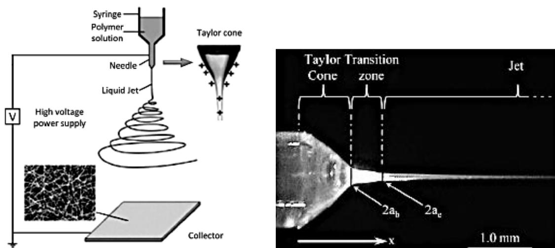
**Figure 13.** Scheme showing the electrospinning process with the Taylor cone on the left, and detail of the Taylor cone zone and the transition zone supporting the fiber formation on the right [63].
