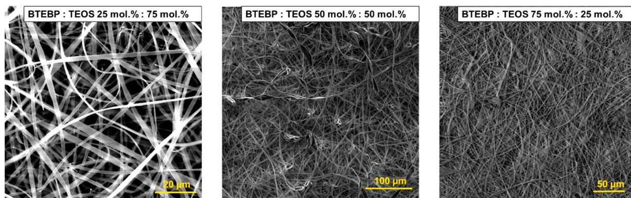
**Figure 41.** SEM images of the prepared BTEBP fibers at different molar ratios.
