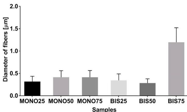
Fig. 5. Fiber diameter with the standard deviation of each material prepared by electrospinning under different operational conditions producing fine smooth fibers: MONO25; MONO50; MONO75; BIS25; BIS50; BIS75.
