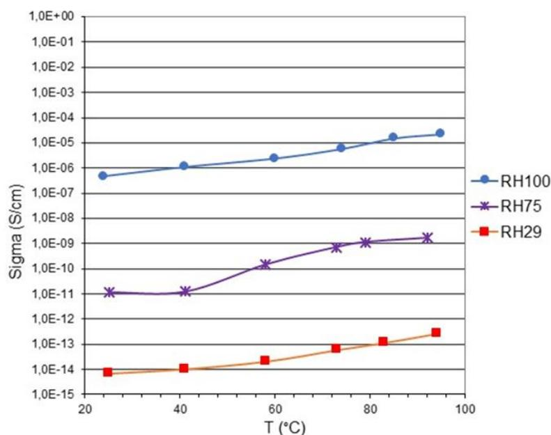
**Figure 44.** Dependence of the specific electrical conductivity on the temperature and relative humidity (RH = 29; 75 and 100) of the environment of hybrid pure organosilane fibers with a BTEBP:TEOS molar ratio of 25 mol. %:75 mol. %.
