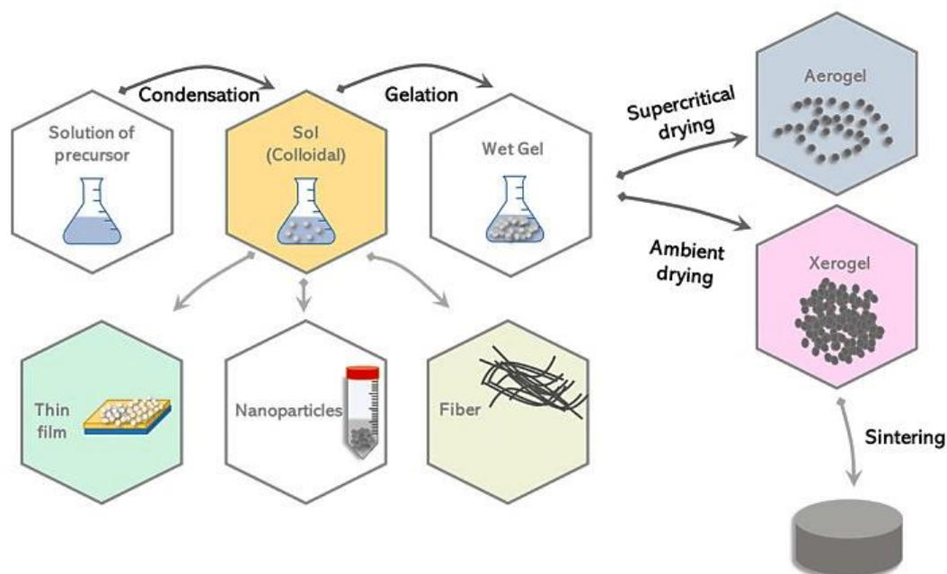
**Figure 6.** Various products, including fibers, that may be obtained using the sol-gel process [47].
