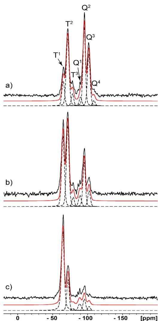
**Figure S1.** Experimental  $^{29}\text{Si}$  CP/MAS NMR spectra (black solid line), simulations of the individual Si atoms (black dashed lines), and their sum (red solid line) of fibrous samples BTEBP 25 mol.% (a); BTEBP 50 mol.% (b), BTEBP 75 mol.% (c).
