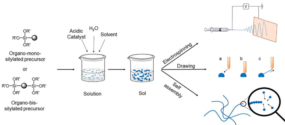
Fig. 5. Preparation of nanofibers from organo-mono-silylated and/or organo-bis-silylated precursors using various fiber making techniques.
