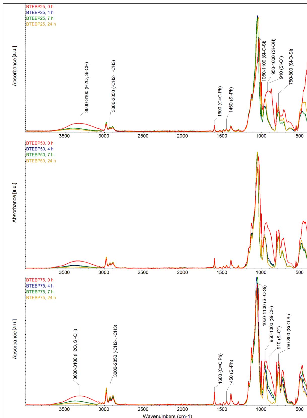
**Figure 36.** FTIR spectra describing the kinetics of the sols containing BTEBP in different molar ratios, which were specified as suitable for the formation of fibers after the established time interval.
