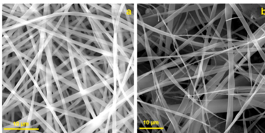
Fig. 14. Electron microscopy images showing organosilane nanofibers prepared from a combination of 1,4-Bis(triethoxysilyl)benzene with TEOS - sample a), and nanofibers prepared from a (1S,2S)-cyclohexane-1,2-diamine-bis-silylated precursor in combination with TEOS - sample b).
