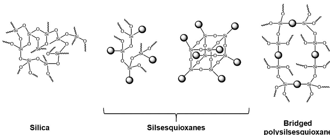
**Figure 3.** Selected organosilane precursors transforming into nets during polycondensation processes. Pure silica is included for comparison [19].
