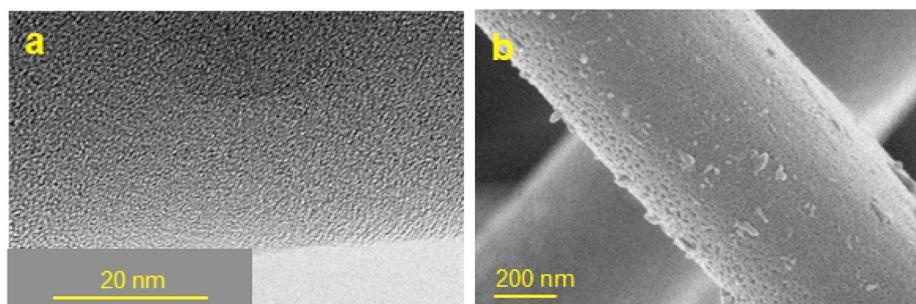
Fig. 6. Sample MONO75 and its microporosity analyzed via TEM a); sample BIS75 showing mesopores in its structure visible by SEM b).
