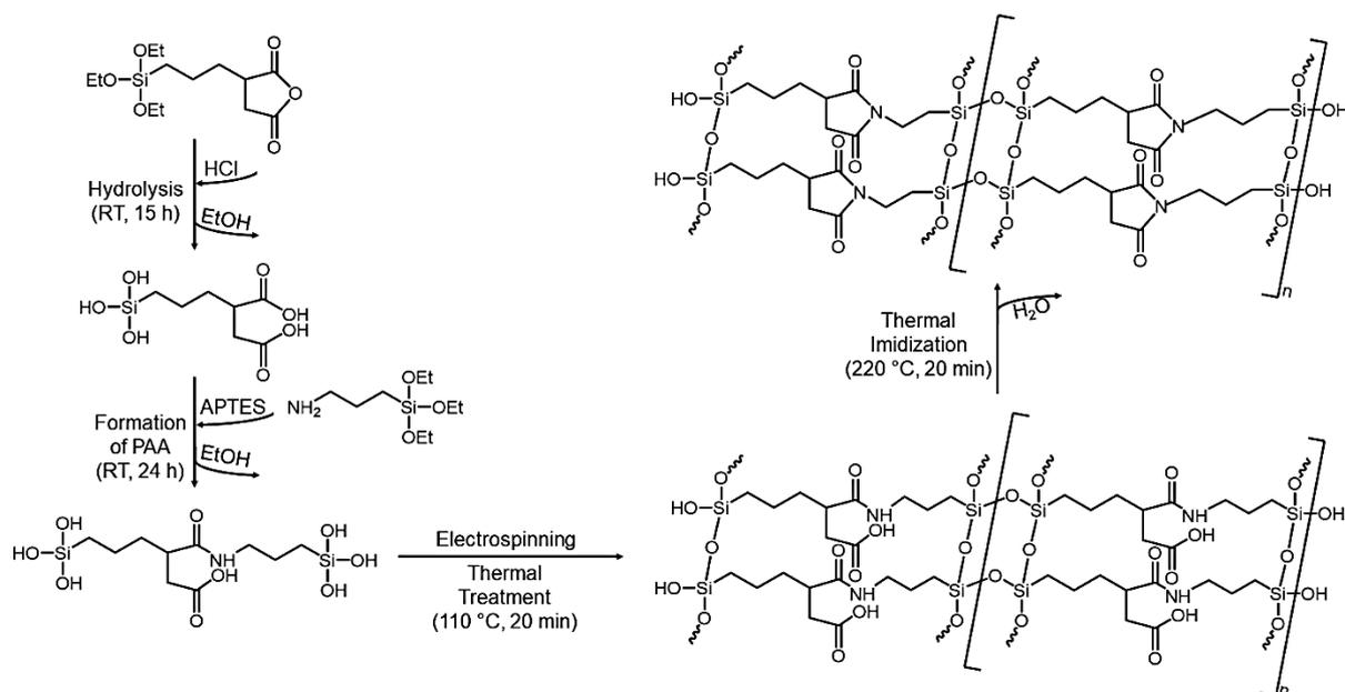
**Figure 19.** Schematic representation of the preparation of polyimide-silane fibers [121].
