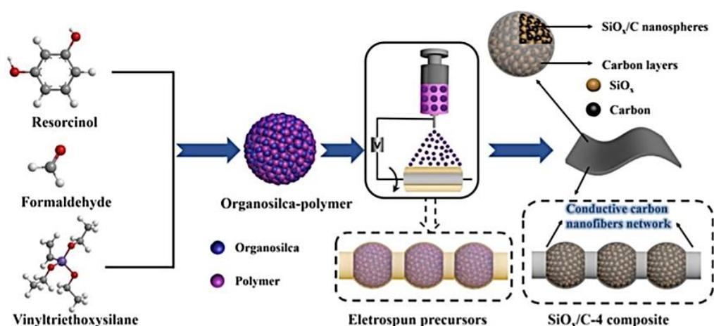
**Figure 28.** A scheme showing the design of the pea-pod structure of  $\text{SiO}_x/\text{C}$  nanofibers [149].
