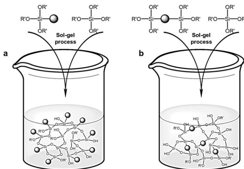
**Figure 10.** Scheme describing the polycondensation processes of **a)** organo-mono-silylated and **b)** organo-bis-silylated precursors [19].
