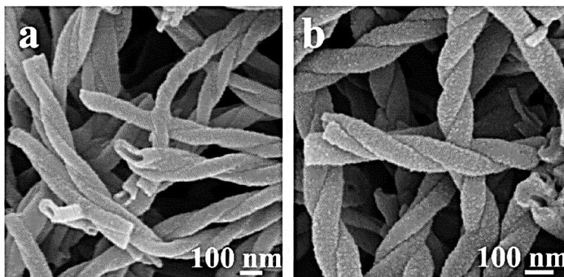
**Figure 35.** FESEM images of (a,b) showing formation of 4,4'-biphenylene bridged polybissilsesquioxane nanotubes via self-assembly [98].
