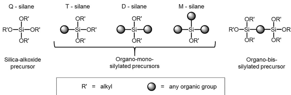
**Figure 2.** Scheme showing the different types of organosilanes [19].
