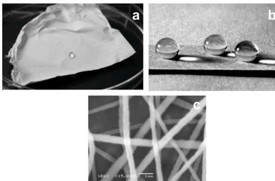
**Fig. 6.** Free-standing mat composed of PS-PDMS/PS electrospun fibers **a**); several 20 µL water droplets on the mat, showing a superhydrophobic surface **b**); SEM image of the prepared fibers at 6000x magnification (scale bar = 2 µm) **c**); [86].
