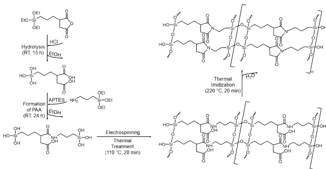
Fig. 9. Schematic representation of the preparation of polyimide-silane fibers, adapted according to reference [105].
