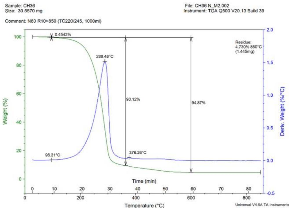
**Figure 47.** TGA spectrum determining the thermal stability of the OBA precursor in the range of 10 to 800 °C.
