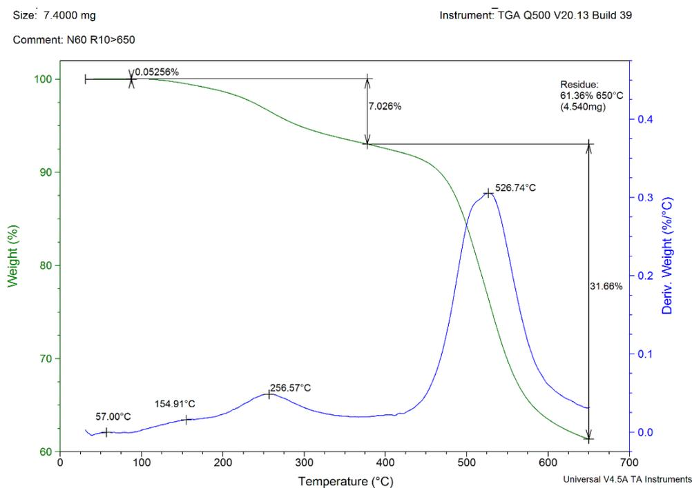
**Figure 40.** TGA spectrum of the thermal decomposition of the organosilane fibers containing BTEBP (75 mol.%) in the hybrid network. The temperature range moves between 25 and 650 °C.
