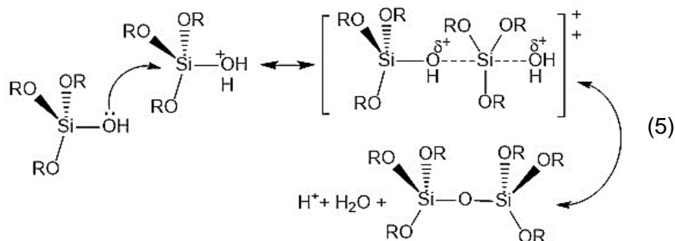
**Figure 9.** Scheme showing the nucleophilic attack of the neutral silanol on the acid-protonated silanol to again give the pentacoordinated intermediate.
