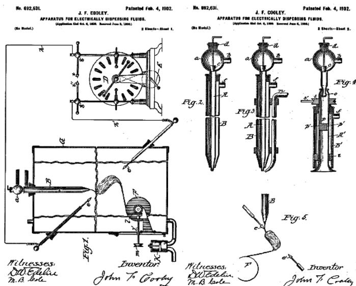
**Figure 12.** US Patent #692631 filed by John Francis Cooley in 1902 describing his electrospinning device [64].
