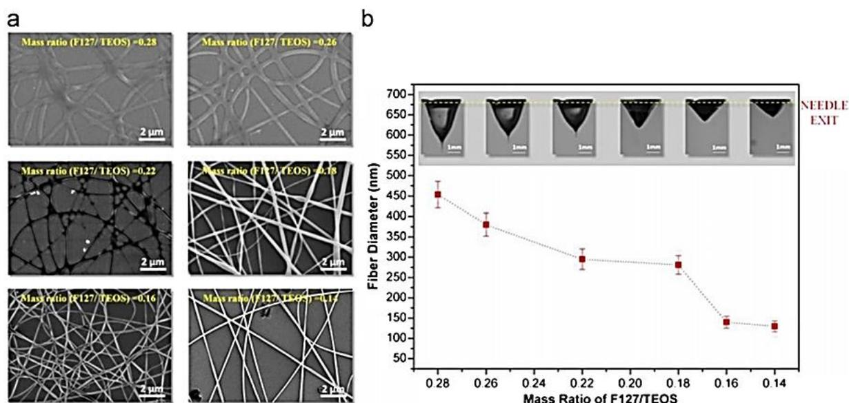
**Figure 21.** SEM images of silica nanofibers prepared using sols with different F127/TEOS mass ratios **a**); and the relationship between the fiber diameter and the F127/TEOS mass ratios **b**); [123].
