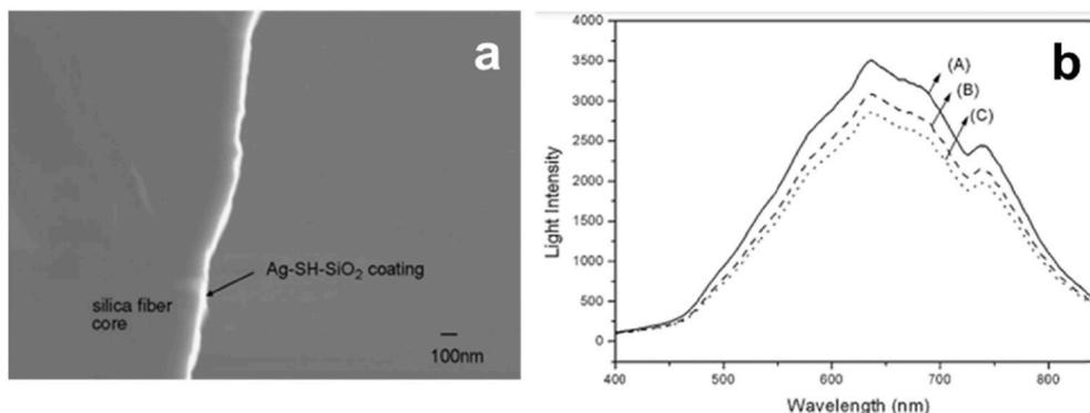
Fig. 8. A SEM image of the cross-section of an optical fiber coated via MPTMS containing Ag nanoparticles and its changes in light intensity guided through the coated fiber probe [92].
