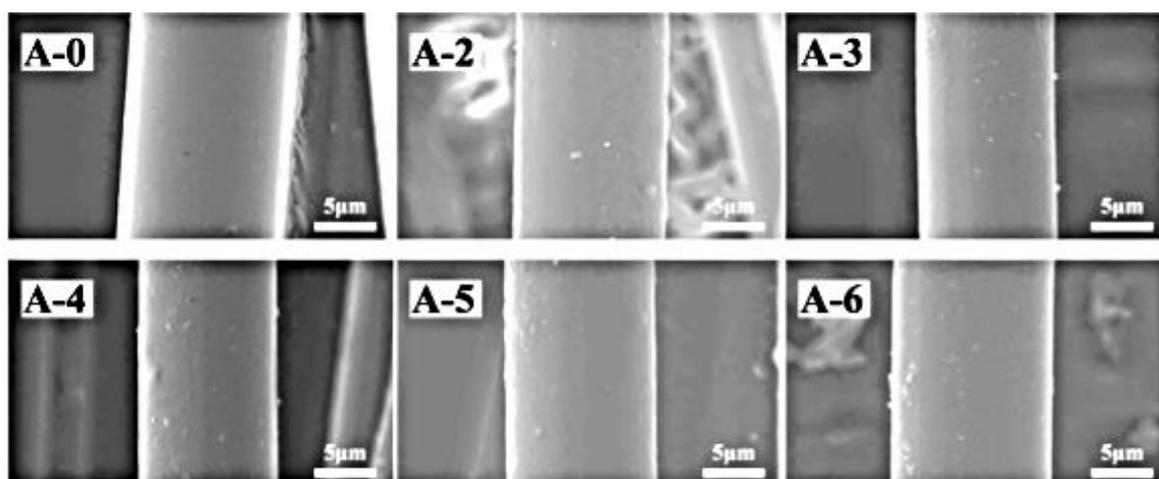
**Figure 26.** SEM images of PI fibers treated with 0, 2, 3, 4, 5 and 6 wt% of APTES (KH-550) [146].
