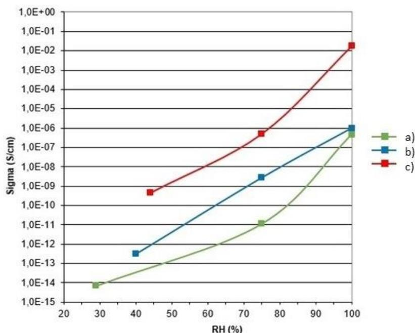
**Figure S3.** The dependence of specific electrical conductivity on the relative humidity of the environment of hybrid pure organosilane fibers **a)** with molar ratio of BTEBP:TEOS 25 mol.% : 75 mol.%; **b)** with a molar ratio of triethoxyphenyl silane (TEPS):TEOS in the sol of 75
