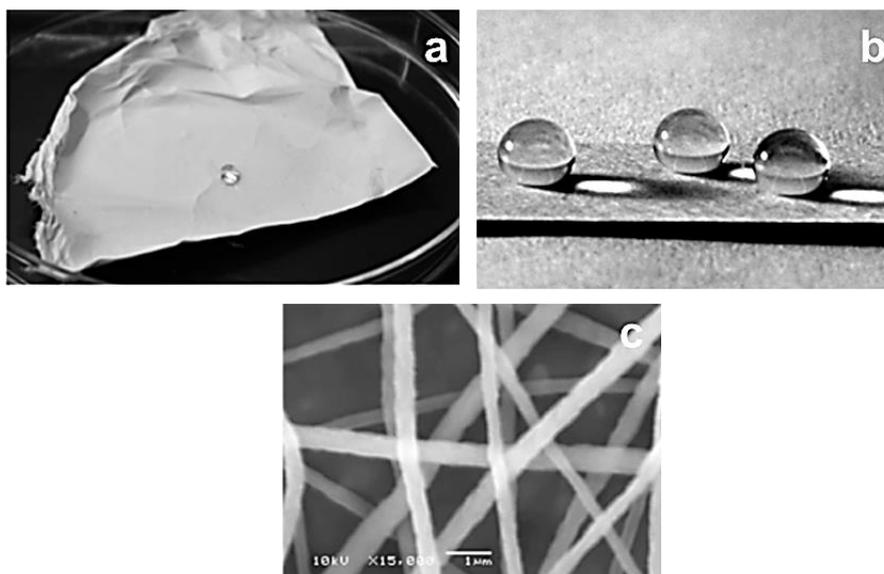
**Figure 16.** Free-standing mat composed of PS-PDMS/PS electrospun fibers **a**); several 20  $\mu\text{L}$  water droplets on the mat, showing a superhydrophobic surface **b**); SEM image of the prepared fibers at 6000x magnification (scale bar = 2  $\mu\text{m}$ ) **c**); [102].
