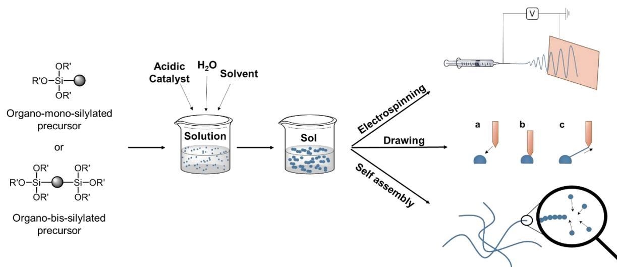
**Figure 11.** Preparation of nanofibers from organo-mono-silylated and/or organo-bis-silylated precursors using various fiber making techniques [19].
