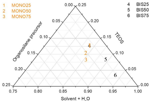
**Fig. 2.** Organosilane precursor, TEOS, and solvent +  $\text{H}_2\text{O}$  molar compositional relationship of the presented organosilane fibers.
