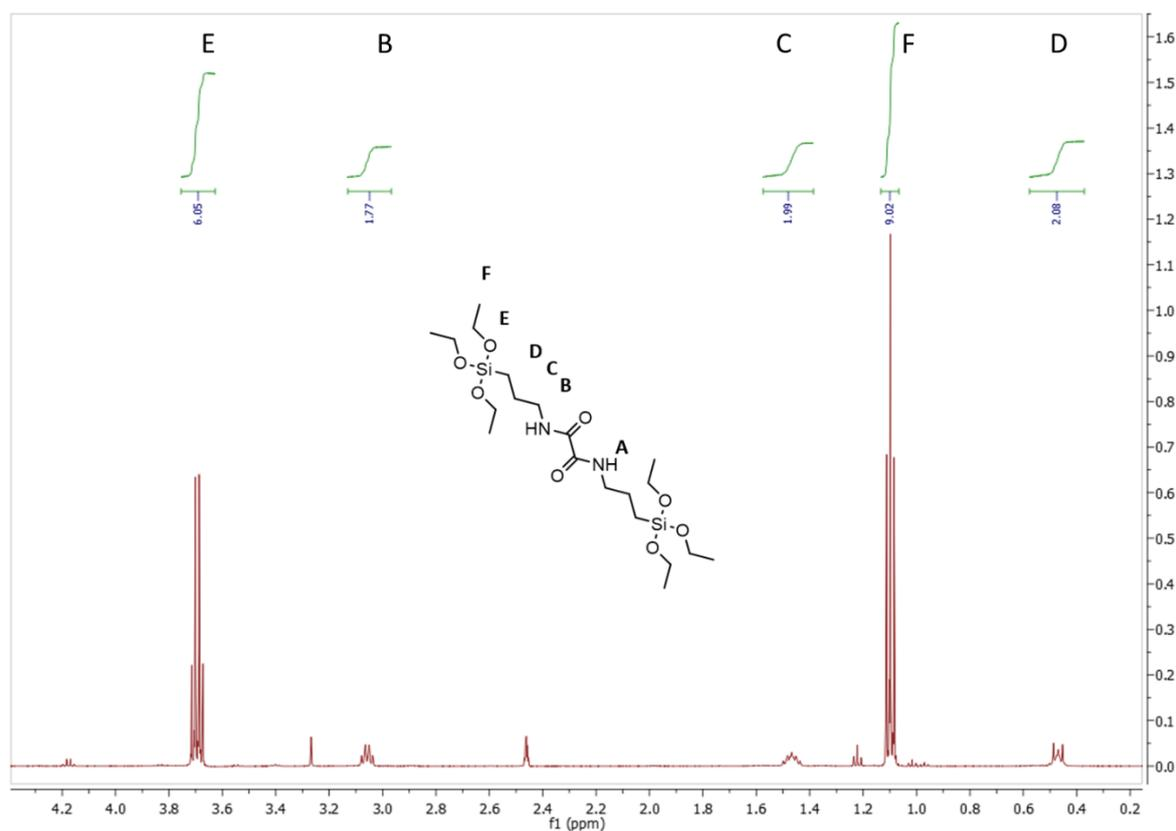
**Figure 45.** Spectrum of the <sup>1</sup>H liquid state NMR of the OBA precursor measured in DMSO-d<sub>6</sub>.
