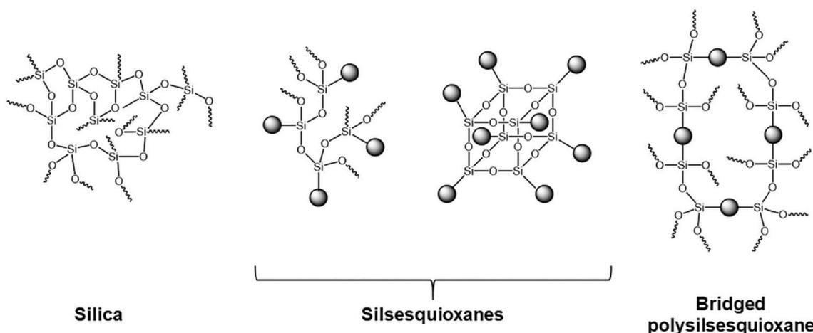
Fig. 3. Selected organosilane precursors transforming into nets during polycondensation processes. Pure silica is included for comparison.
