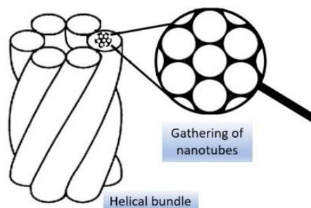
**Figure 25.** Schematic representation of right-handed helical nanofibers[19].
