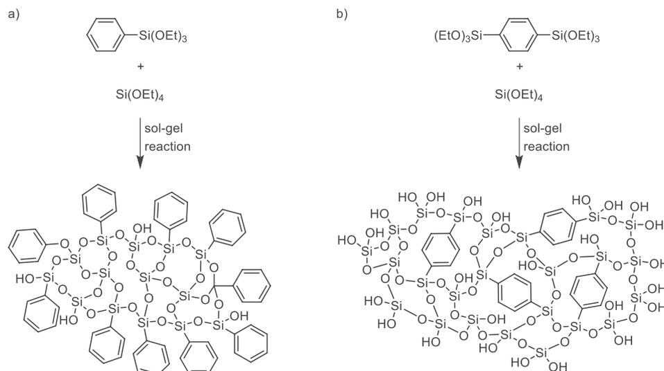
**Fig. 1.** The role of organically functionalized trialkoxysilanes in the silicon-based sol-gel process [1]: a) use of organo-mono-silylated precursors; b) use of bridged organo-bis-silylated precursors.
