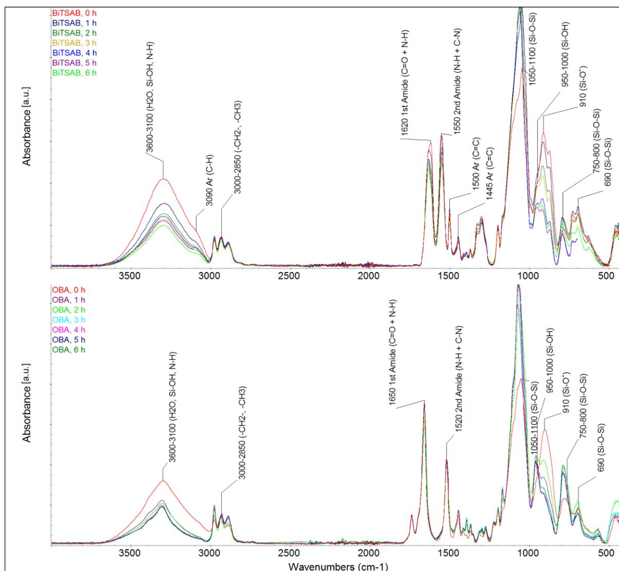
**Figure 49.** FTIR spectra describing the kinetics of the sols containing 50 mol.% of BiTSAB precursor (**upper spectrum**) and OBA precursor (**lower spectrum**) which were established as being suitable for the formation of fibers after 6 hours of heating at an appropriate temperature.
