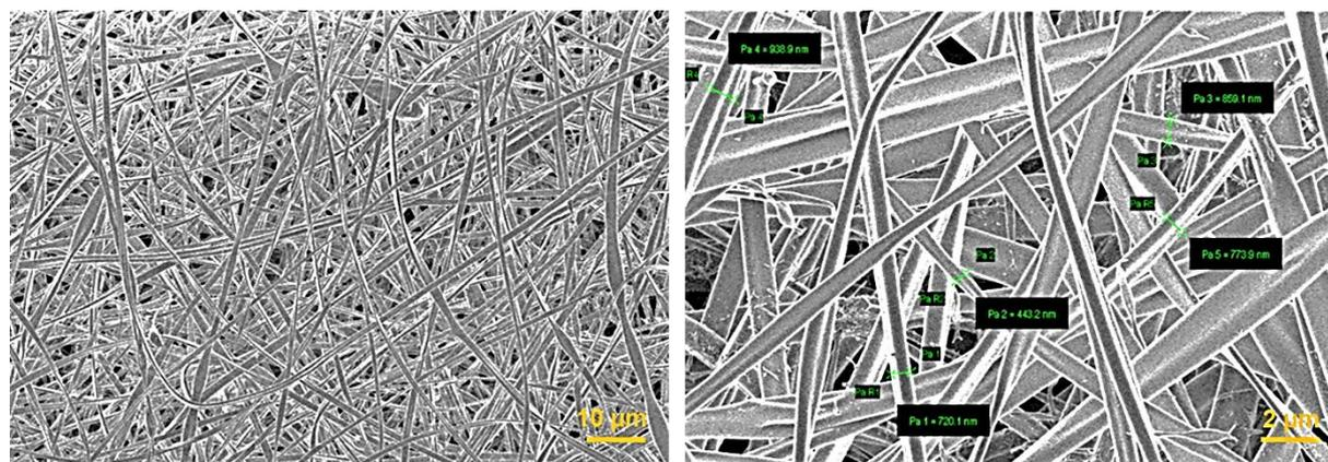
**Figure 51.** Hybrid organosilane fibers prepared from the OBA precursor at 100 mol.% without the use of TEOS.
