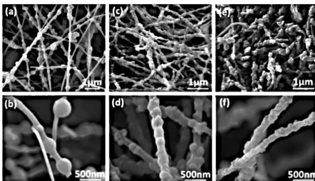
**Figure 29.** SEM images showing the pea-pod structure of  $\text{SiO}_x/\text{C}$  nanofibers with different amounts of  $\text{SiO}_x$  ( $\text{SiO}_x/\text{C}$ -0.3g (**a,b**);  $\text{SiO}_x/\text{C}$ -0.4g (**c,d**) and  $\text{SiO}_x/\text{C}$ -0.5g (**e,f**)) [149].
