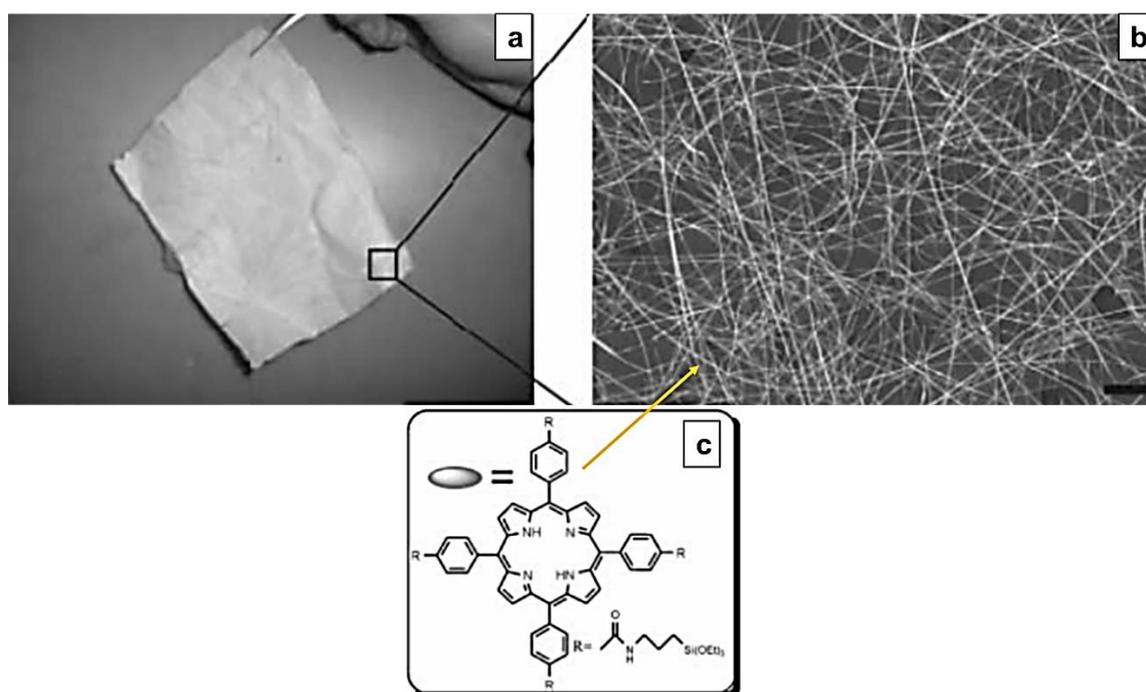
**Figure 30.** Photo of an electrospun porphyrin-doped freestanding nanofibrous membrane **a**); SEM image of this membrane, scale bar = 20 μm **b**); structure of the porphyrin-silane precursor used in the silica matrix with a content of (10<sup>-4</sup> mol.%) **c**)[130].
