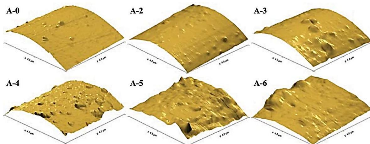
**Figure 27.** AFM images representing PI fiber surface roughness treated with 0, 2, 3, 4, 5 and 6 wt% of APTES (KH-550) [146].
