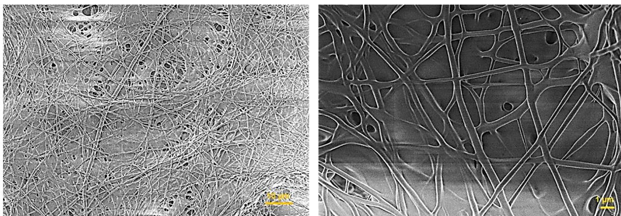
**Figure 50.** Fibers prepared from a combination of the OBA precursor:TEOS 50 mol.%
