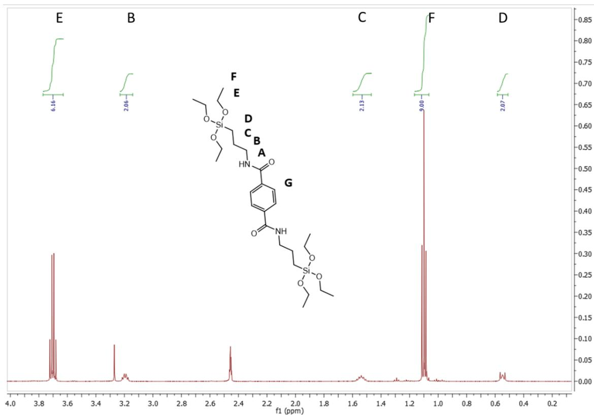
**Figure 46.** Spectrum of the  $^1\text{H}$  liquid state NMR of the BiTSAB precursor measured in  $\text{DMSO-d}_6$ .
