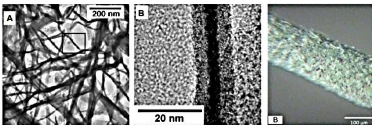
**Figure 31.** Si<sub>2</sub>-Pt nanofibers containing Pt nanocrystals **a**); HRTEM image of the boxed region in Figure 32a **b**) - center [165]; optical microscopic image of a proposed SPME fiber **b**) - right [166].
