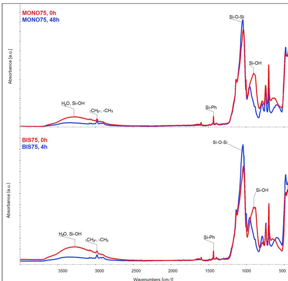
Fig. 3. FTIR spectra of the MONO75 and BIS75 sols at the beginning and at the end of the sol-gel process.
