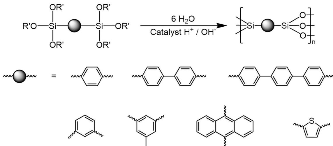
Fig. 12. Representatives of arylene bridged polysilsesquioxanes.
