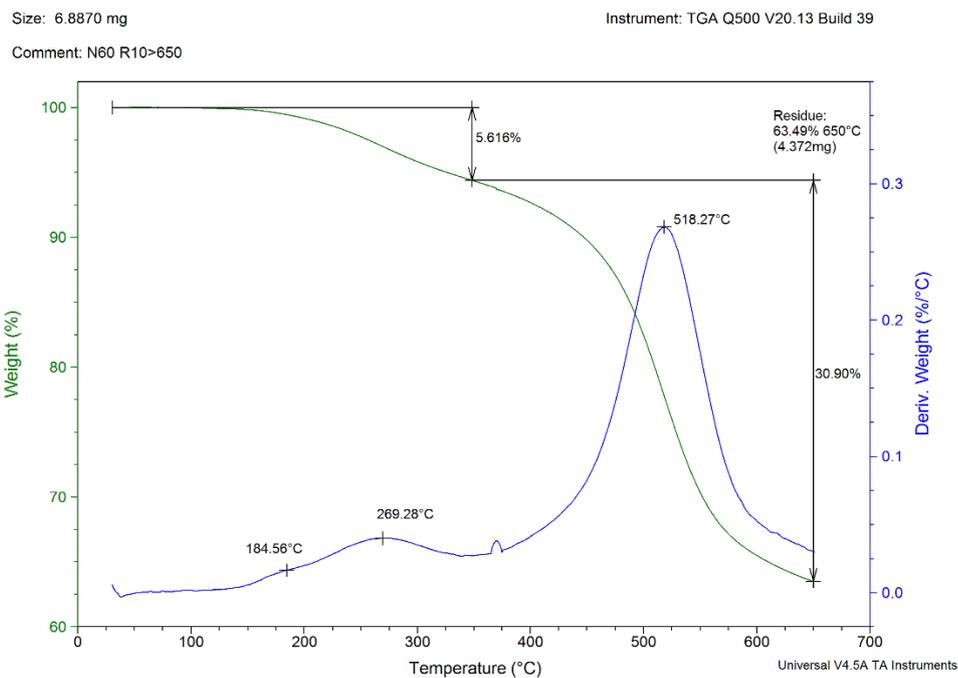
**Figure 39.** TGA spectrum of the thermal decomposition of the organosilane fibers containing BTEBP (50 mol.%) in the hybrid network. The temperature range moves between 25 and 650 °C.
