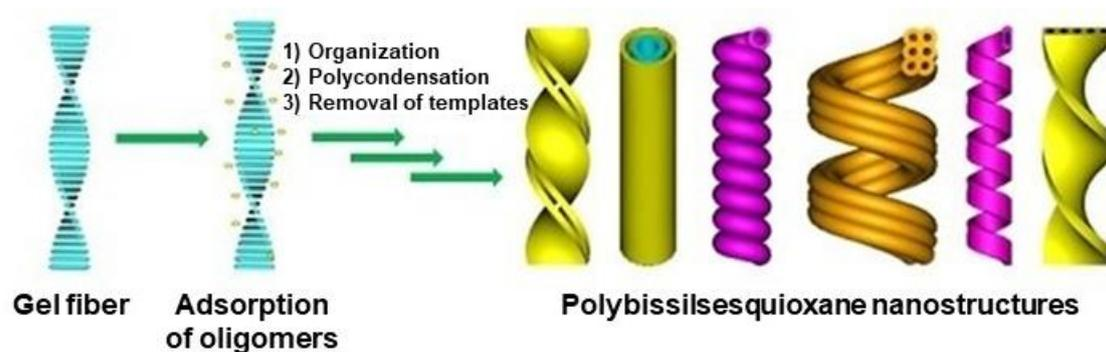
**Figure 15.** Scheme demonstrating the formation of single-handed helical polybissilsesquioxane nanostructures in the form of mesoporous nanofibers by self-assembly [98].
