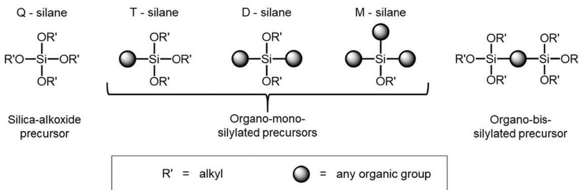
Fig. 2. Scheme showing the different types of organosilanes.
