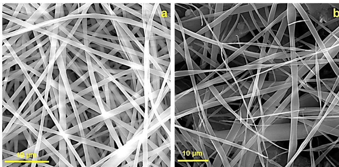
**Figure 23.** Electron microscopy images showing organosilane nanofibers prepared from a combination of 1,4-bis(triethoxysilyl)benzene with TEOS - sample **a**), and nanofibers prepared from a (1*S*,2*S*)-cyclohexane-1,2-diamine – bis – silylated precursor in combination with TEOS - sample **b**) [19,132].
