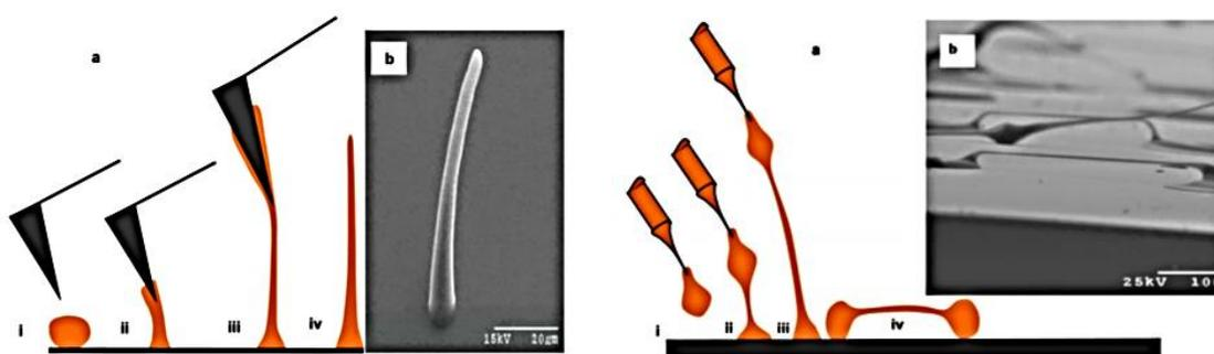
**Figure 14.** Fiber drawing based on the AFM/STM probe **a**); SEM image of a drawn vertical fiber **b**) – left image. Process of micro-pipette probe fiber drawing **a**); SEM image of a suspended fiber **b**) – right image [76].
