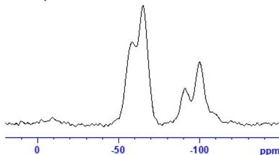
Figure 4. <sup>29</sup>Si CP/MAS NMR spectra of the hybrid DACHsilane fibres.
