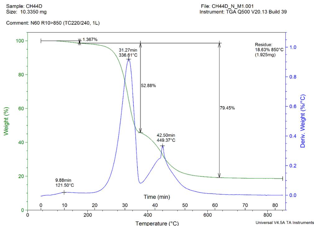
**Figure 48.** TGA measurement determining the thermal stability of the BiTSAB precursor in the range of 10 to 800 °C
