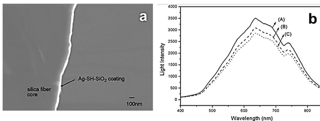
**Figure 18.** A SEM image of the cross-section of an optical fiber coated via MPTMS containing Ag nanoparticles and its changes in light intensity guided through the coated fiber probe [108].
