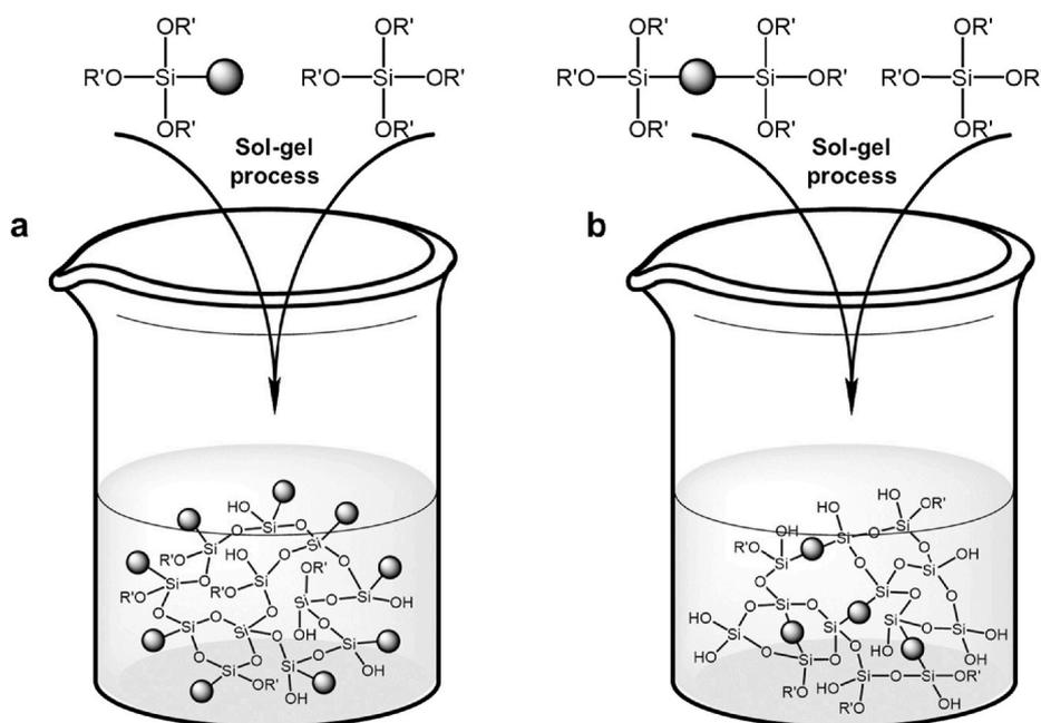
Fig. 4. Scheme describing the polycondensation processes of organo-mono-silylated a) and organo-bis-silylated precursors b).
