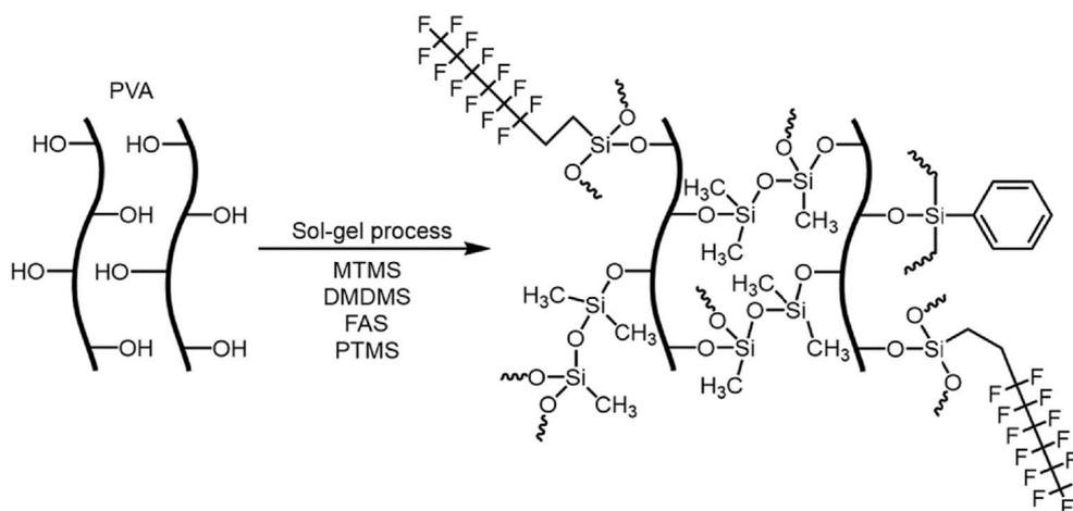
Fig. 7. Scheme of PVA/silica nanofibrous mats, adapted according to reference [88].
