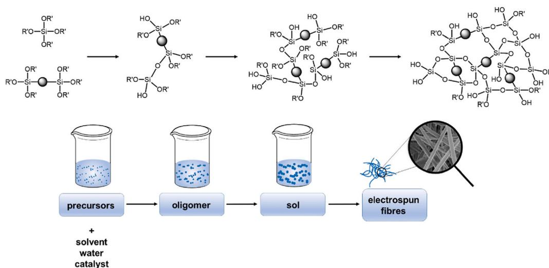
Fig. 13. General scheme of the use of any organo-bis-silylated precursor leading to the formation of organosilane fibers.
