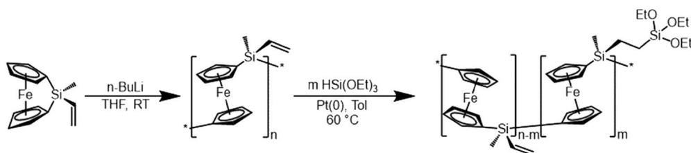
Fig. 10. Scheme showing the formation of an organo-mono-silylated precursor, adapted according to reference [106].
