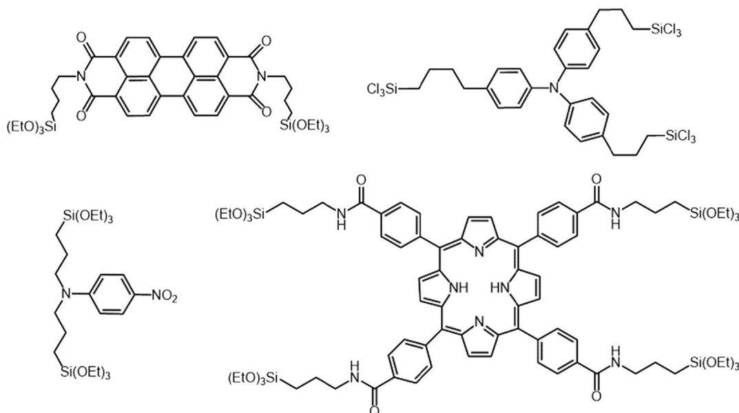
**Fig. 18.** Examples of bridged polysilsesquioxanes with chromophore bridging groups, adapted according to reference [39].
