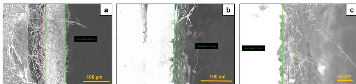
**Figure 43.** SEM images showing the layer thickness ( $\mu\text{m}$ ) of the prepared hybrid organosilane BTEBP fibers at various molar ratios (BTEBP 25 mol.% **a**); BTEBP 50 mol.% **b**); BTEBP 75 mol.% **c**).
