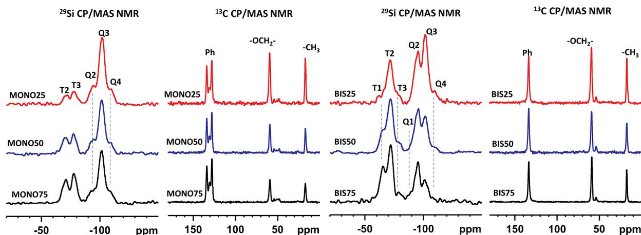
Fig. 7.  $^{29}\text{Si}$  CP/MAS and  $^{13}\text{C}$  CP/MAS NMR spectra of the investigated samples MONO25, MONO50, MONO75 a); and samples BIS25, BIS50, BIS75 b).
