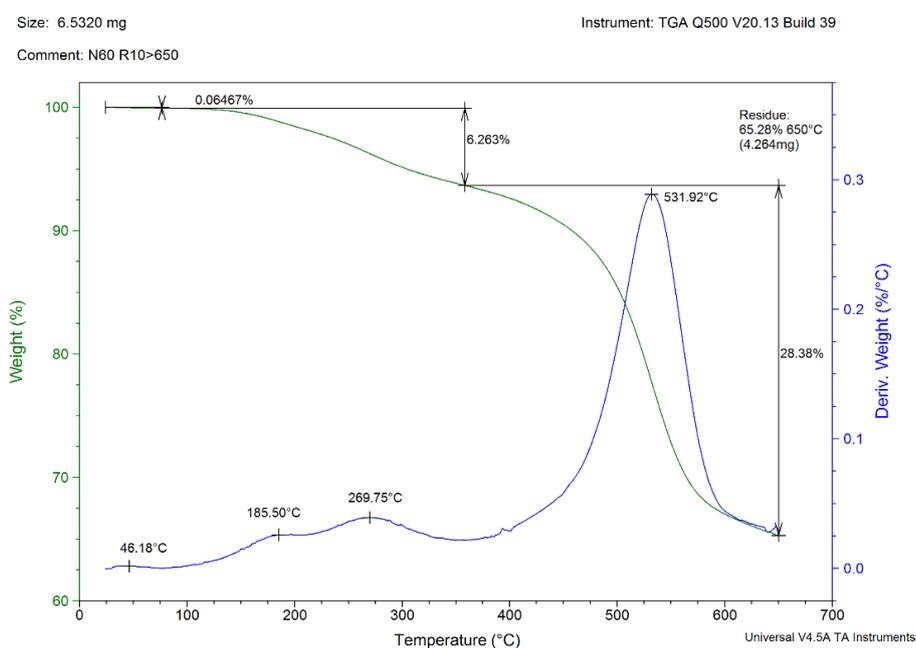
**Figure 38.** TGA spectrum of the thermal decomposition of the organosilane fibers containing BTEBP (25 mol.%) in the hybrid network. The temperature range moves between 25 and 650 °C.
