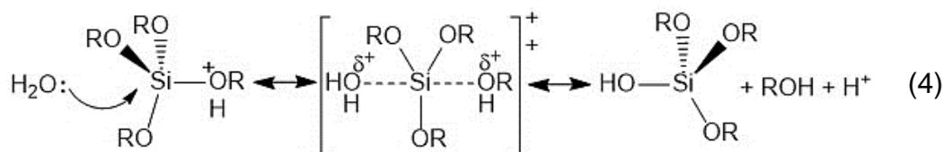
**Figure 8.** Scheme showing the formation of the pentacovalent intermediate on the silicon atom.
