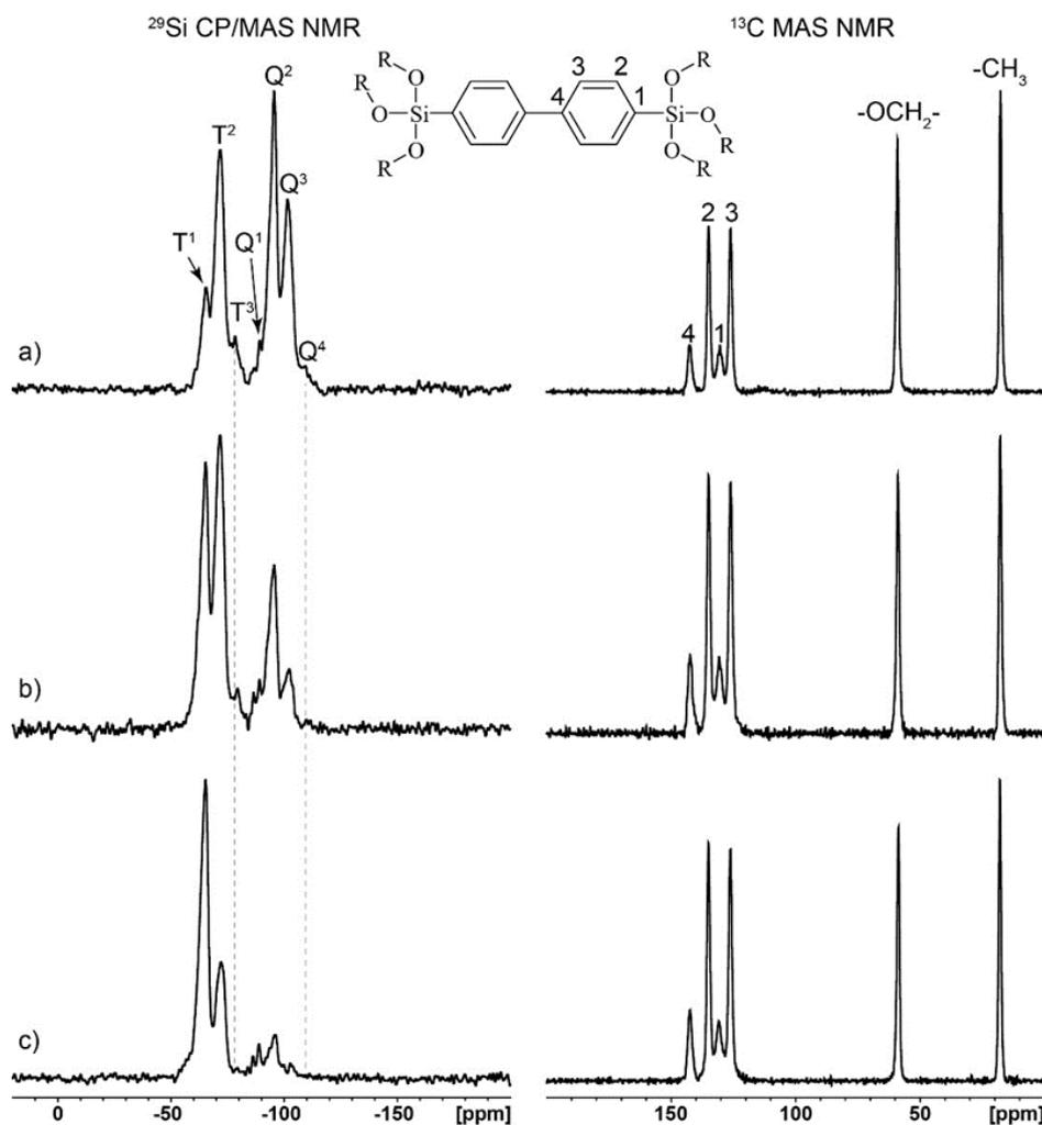
**Figure 37.** ssNMR spectra of the fibers: **a)** variant with a molar ratio of BTEBP:TEOS 25 mol.:%:75 mol.%; **b)** variant with a molar ratio of BTEBP:TEOS 50 mol.:%:50 mol.%; **c)** variant with a molar ratio of BTEBP:TEOS in the sol of 75 mol.:%:25 mol.%.
