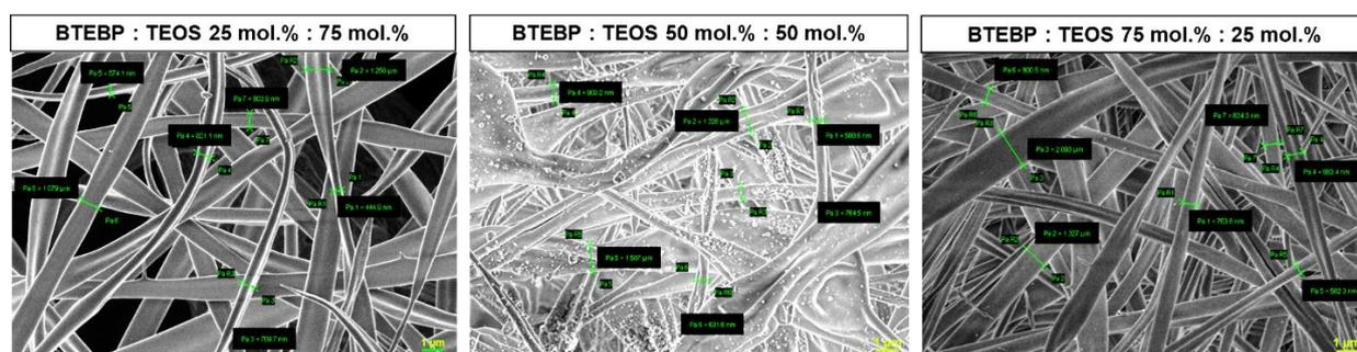
**Figure 42.** SEM images showing the diameters of the prepared hybrid organosilane BTEBP fibers.
