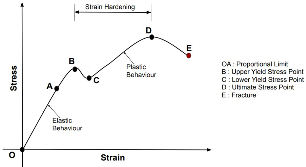
Figure 8 - Stress-strain curve [34]
