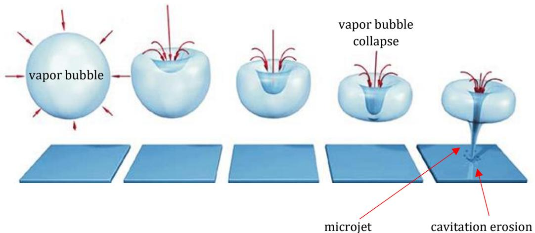
Figure 3 - Formation of cavitating microjet [37]
