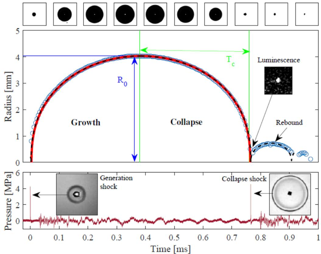
*Figure 4 – Multiple phenomena presented, with collapse shock wave in the bottom of the figure. Top of the figure: shadowgraph visualization of spherical bubble growth and collapse, middle: evolution of a bubble, bottom: pressure signal as a function of time [11]*
