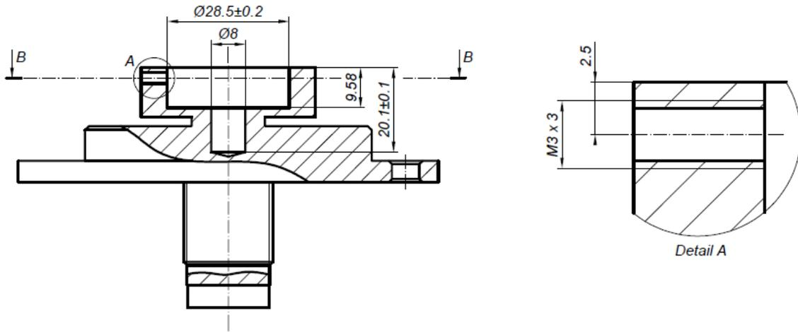
Figure 14 - Side view of holder with detail A
