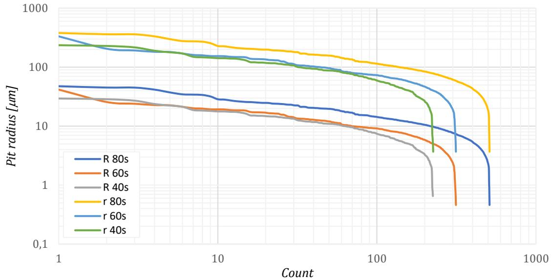
Figure 20 - Graphical representation of relation between real and measured damage size
