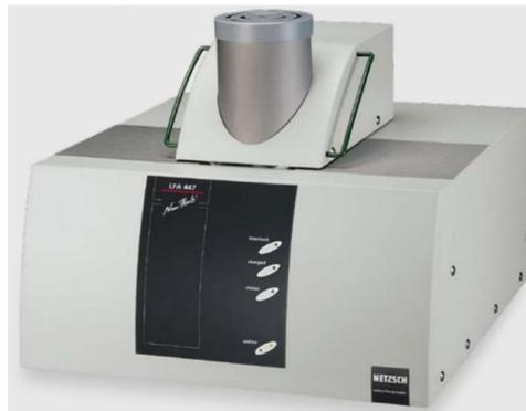
Fig. 4.6 System of thermal conductivity NETZSCH model LFA 447 NanoFlash
