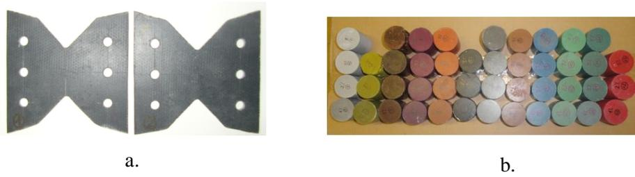
Fig. 6.5 a. Geocomposite samples after cutting and drilling; b. Geopolymer mortar with different colors
