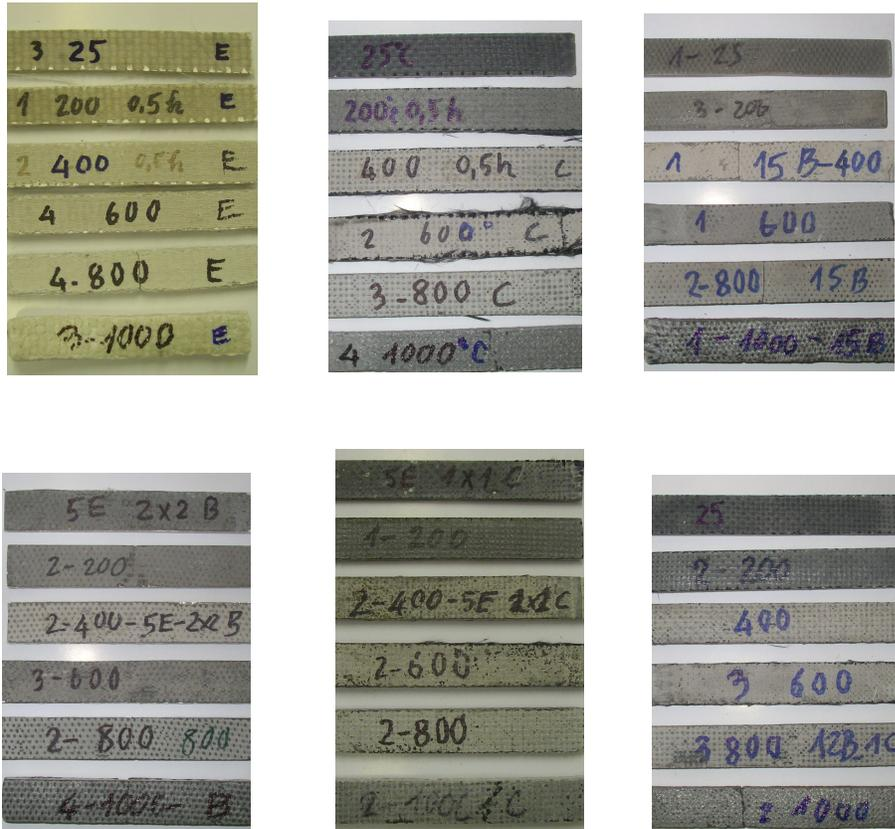
Fig. A.1 Geocomposite samples: 7E, 10C, 15B, 5E+2x2B, 5E+2x1C, 12B+2x1C after heating at different level 200 °C, 400 °C, 600 °C, 800 °C, and 1000 °C for 30 mins.
