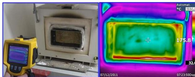
Fig. 6.4 Wooden plate coated by geopolymer mortar (left) and after heated 354 °C in the oven, outside only 175.8 °C
