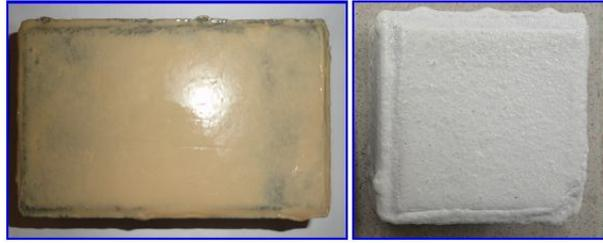
Fig. 6.2 Portland concrete coated by pure geopolymer before (left) and after heated 600 °C (right)
