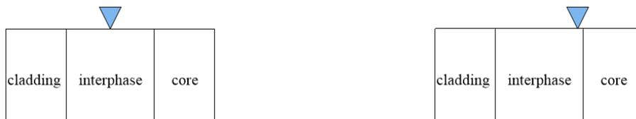
Figure 5.20 Possibilities of one indent with 80 nm depth and 1300 nm spacing in the interphase region.
