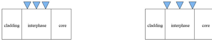
Figure 5.24 Possibilities of three indents with 40 nm depth and 400 nm spacing in the interphase region.
