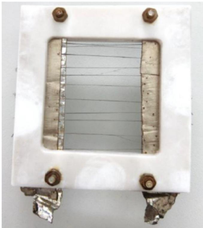
FIGURE 3.2: Polypyrrole-coated PCL fibers made by drawing, fixed within a Teflon frame in between an aluminum foil.
