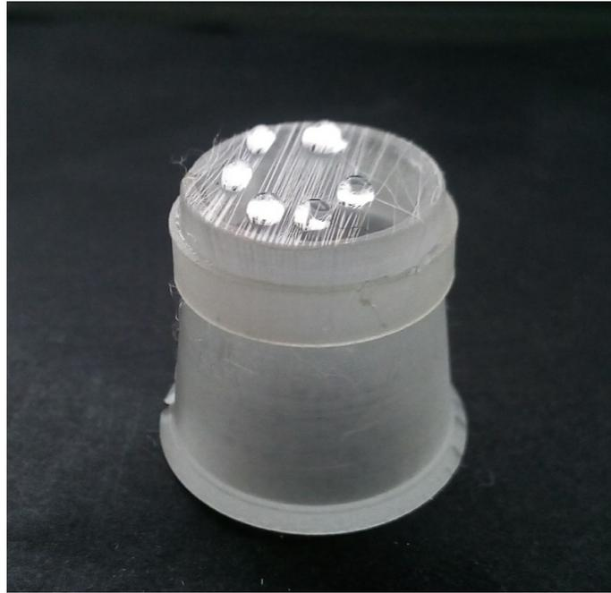
FIGURE 3.1: Measuring the WCA on the drawn samples fixed within the fixation ring.
