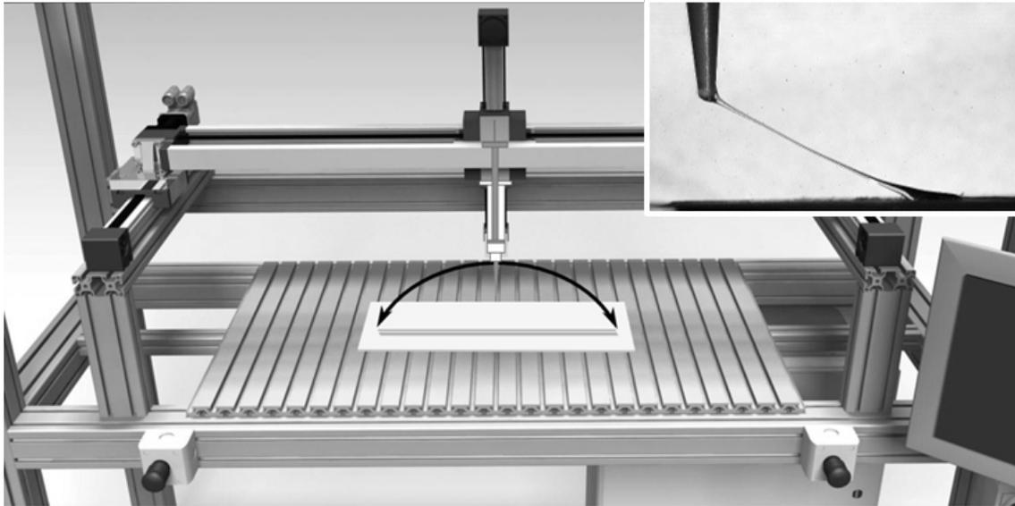
FIGURE 4.1: The manipulator representing the drawing movement (Strnadová et al., 2020)
