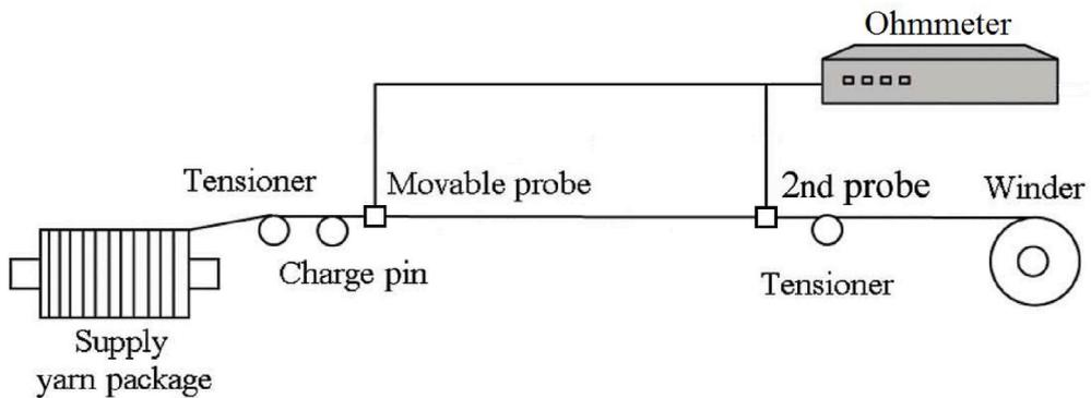
Fig. 5. Configuration of electrical resistance measurement of samples.
