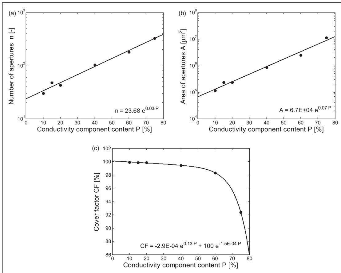
**Figure 6.** The dependence of (a) number of apertures, (b) area of apertures and (c) cover factor on the conductivity component content.
