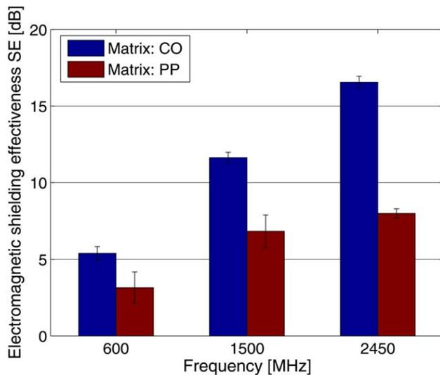
FIG. 12. Comparison of SE of samples with different matrix material (PP, CO) at different frequencies. [Color figure can be viewed at wileyonlinelibrary.com.]
