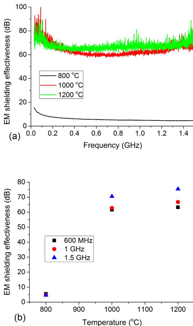
Fig. 12. (a). Effect of frequency on electromagnetic shielding effectiveness. (b). Effect of carbonization temperature on electromagnetic shielding effectiveness in low frequency region. (A colour version of this figure can be viewed online.)
