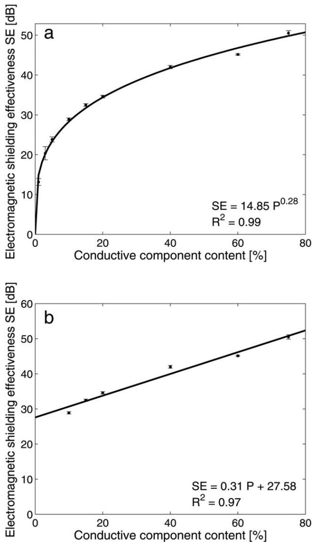
FIG. 6. The dependence of shielding effectiveness on metal fiber content for (a) samples: W1–W75, (b) samples with conductive component above percolation threshold: W10–W75.
