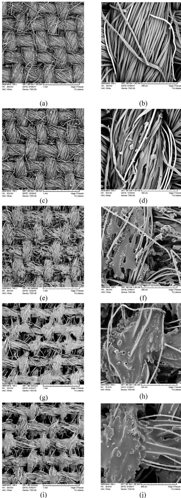
**Fig. 9.** SEM images of: (a and b) untreated sample and laser treated samples with different intensities expressed by gray scale [%]: (c and d) GS 19.2%, (e and f) GS 34.5%, (g and h) 46.7%, (i and j) 56.9%.
