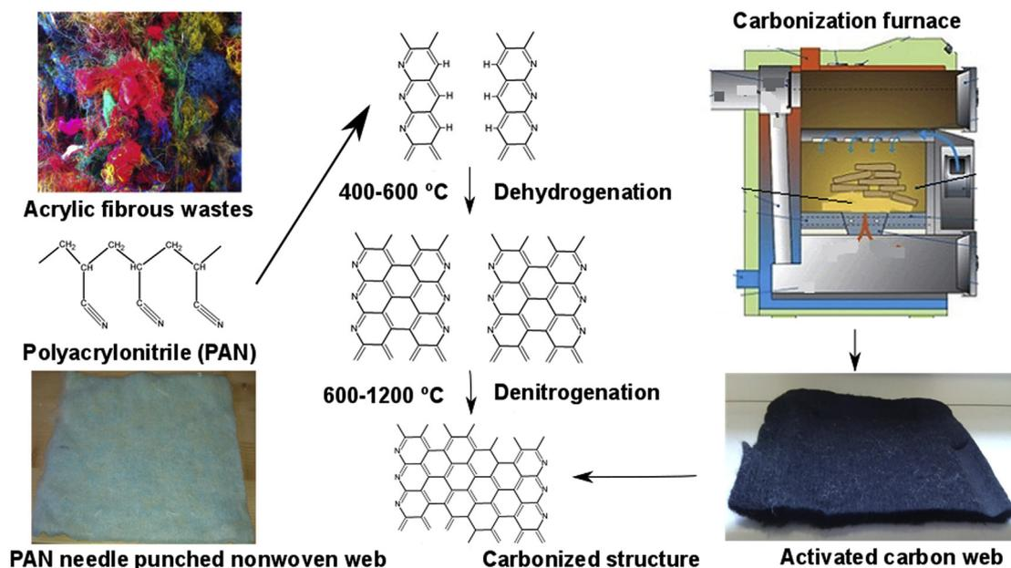
Fig. 1. Schematic of preparation of activated carbon from acrylic fibrous wastes. (A colour version of this figure can be viewed online.)
