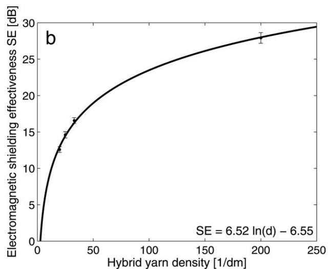
FIG. 11. The dependence of shielding effectiveness on hybrid yarn spacing at (a) 1.5 GHz, (b) 2.45 GHz.
