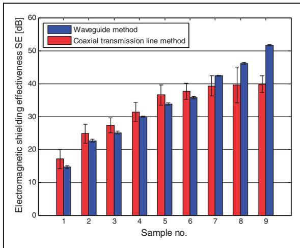
**Figure 6.** Comparison of mean values of SE measured by both methods along with 95 % confidence intervals for mean.
