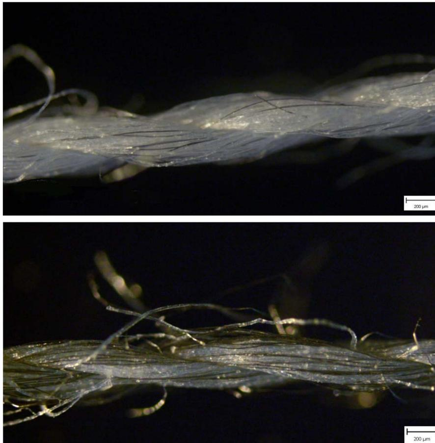
FIG. 1. Microscopic images of two ply hybrid yarns containing (a) 15 %, (b) 60 % of conductive component. [Color figure can be viewed at [wileyonlinelibrary.com](http://wileyonlinelibrary.com)]
