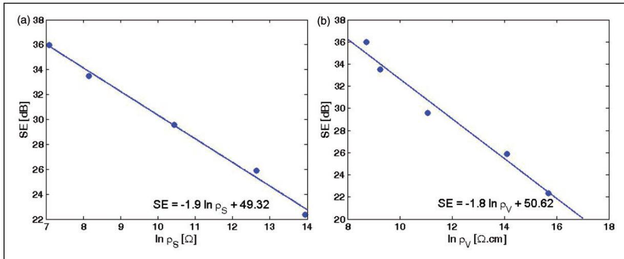
**Figure 7.** The dependence of shielding effectiveness on the logarithm of (a) the surface and (b) volume resistivity in the area above the percolation threshold.
