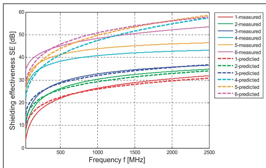
**Figure 8.** Frequency dependence of electromagnetic shielding effectiveness – comparison of predicted and measured values for all samples.
