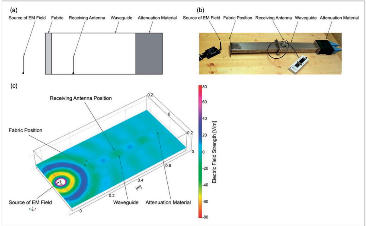
**Figure 1.** (a) The test set-up, (b) image of proposed rectangular waveguide, (c) simulation of electromagnetic wave entering the waveguide.
