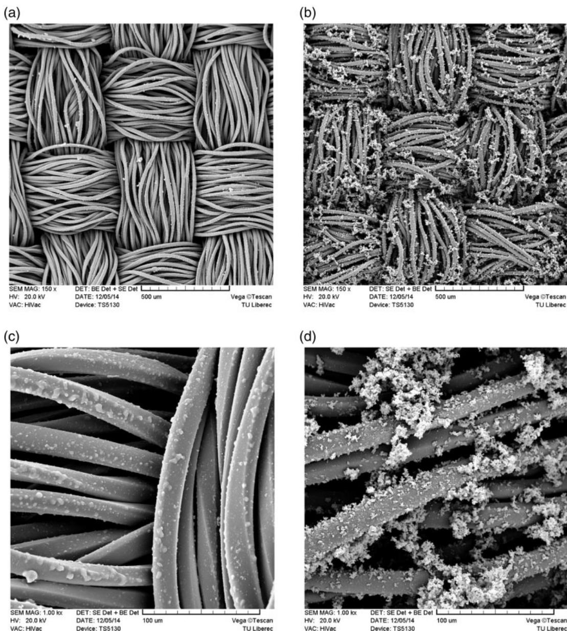
**Figure 10.** SEM pictures of PET/PPy textile composites prepared by following adjustments: (a),(c) 5°C, 1 h, 0.64 g/l, (b),(d) 15°C, 15 h, 5.8 g/l. Two different magnitudes were used: 150× and 1000×.
