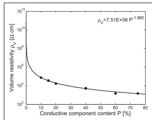
**Figure 3.** The dependence volume resistivity of samples on percentage of conductive component.
