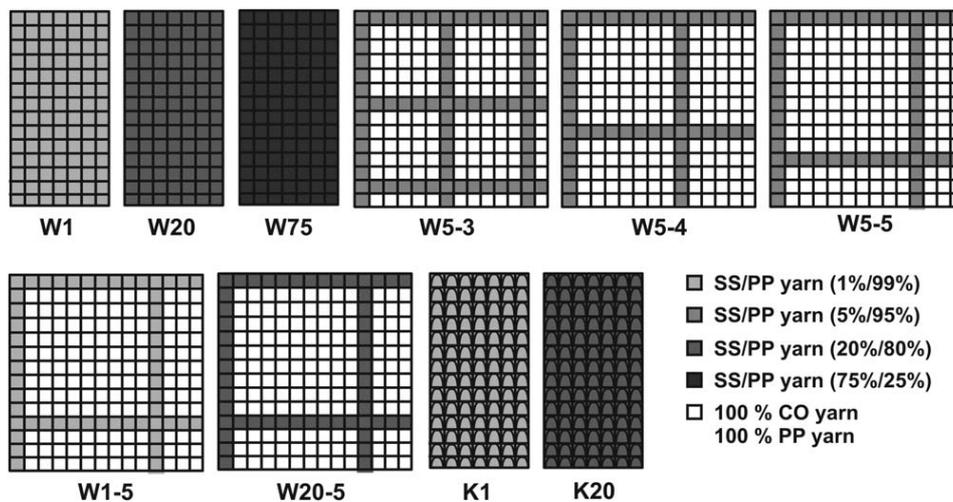
FIG. 2. Schematic diagram of hybrid fabric structure (grey squares: hybrid yarns, white squares: 100 % cotton yarns or 100% polyester yarns).
