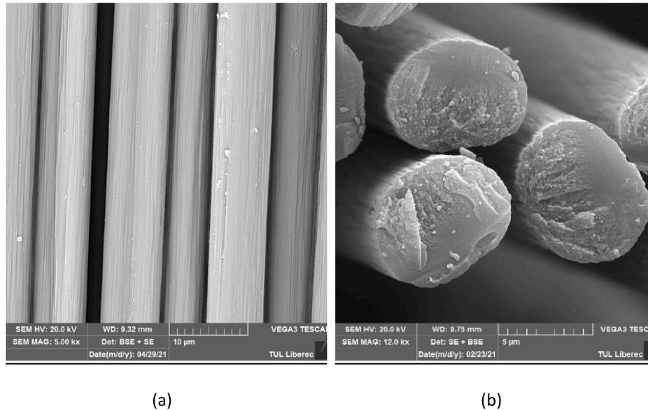
Fig. 2. Microscopic images of the carbon fibers in carbon roving.
