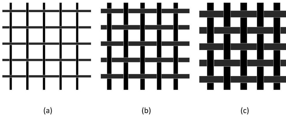
Fig. 4. Schematics of samples with the same roving spacing,  $s = 15$  mm, but different roving diameters: (a)  $2r$ , (b)  $2 \times 2r$ , and (c)  $3 \times 2r$ .
