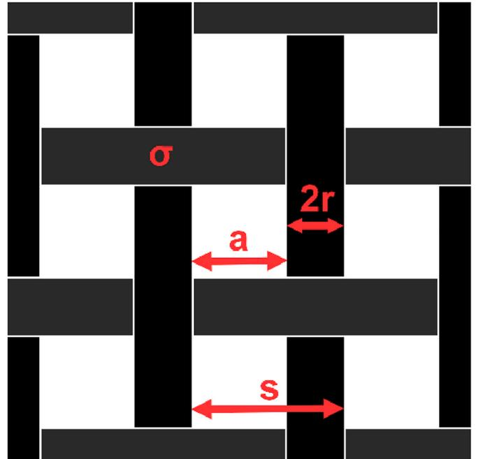
Fig. 1. Planar mesh screen with bonded junctions.
