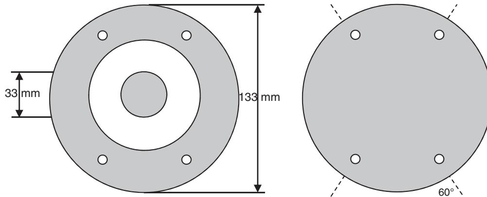
**Figure 2.** Illustrations of (a) reference and (b) load sample for measurement of electromagnetic shielding effectiveness.
