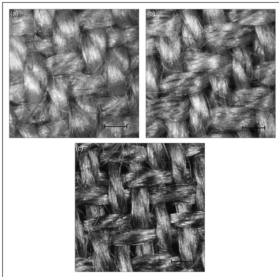
**Figure 3.** Microscopic image of chosen studied fabrics: (a) sample no. 3 (95% PP/ 5% SST), (b) sample no. 6 (80% PP/ 20% SST), (c) sample no. 9 (25% PP/75% SST).
