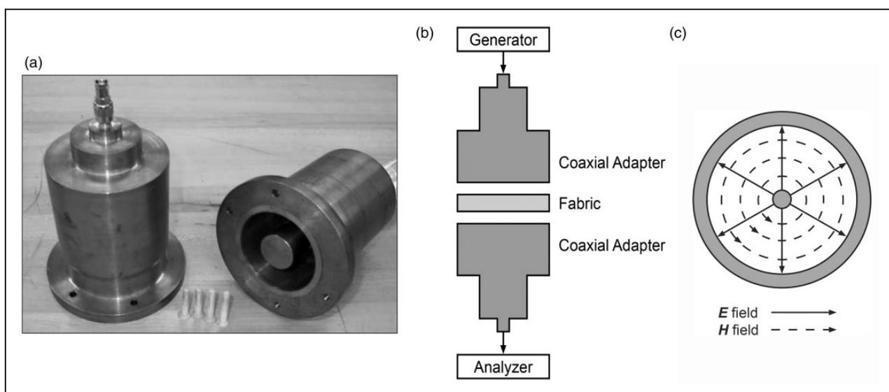
**Figure 4.** (a, b) Set-up with coaxial adapters, (c) electric and magnetic field distribution inside a coaxial line.
