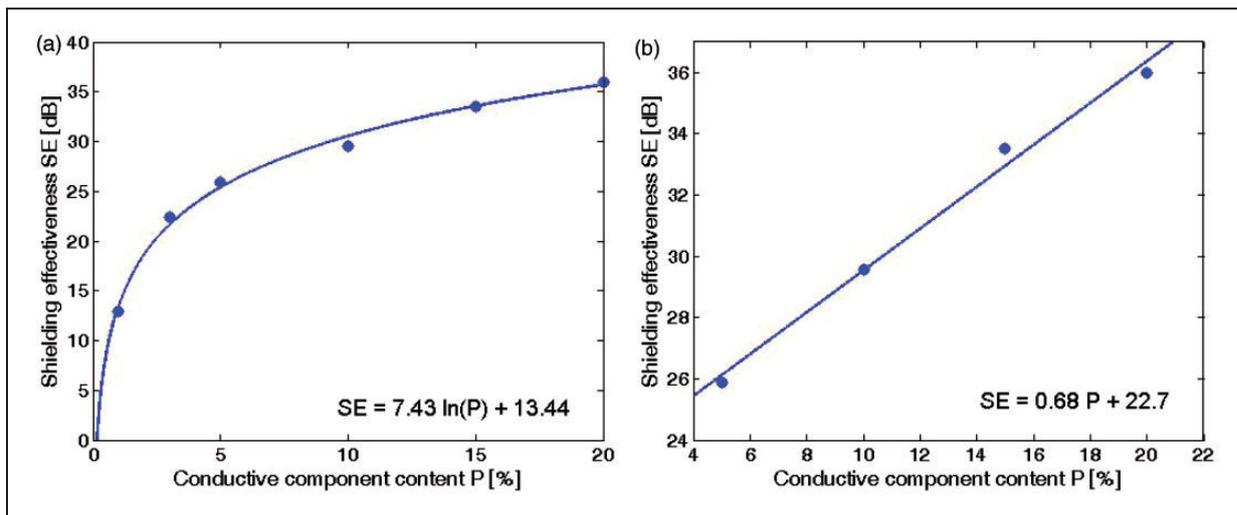
Figure 6. The dependence of shielding effectiveness on conductive component content for (a) the whole range of samples and (b) samples above the percolation threshold.
