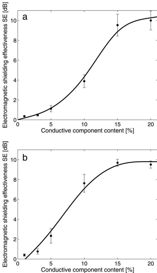
FIG. 8. The dependence of shielding effectiveness on metal fiber content for knitted samples at frequency (a) 1 GHz, (b) 1.5 GHz.
