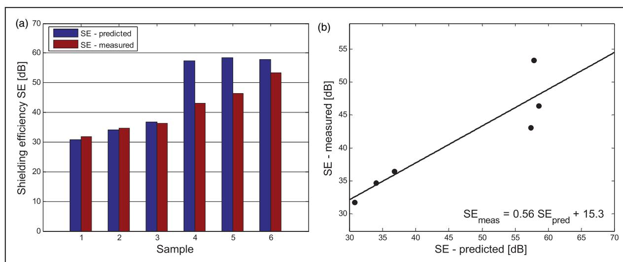
**Figure 9.** (a) comparison of predicted and measured electromagnetic shielding effectiveness for frequency 2450 MHz. (b) empirical Q–Q plot.
