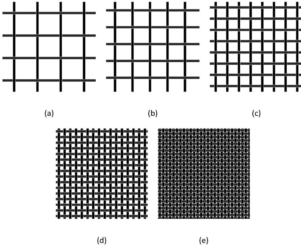
Fig. 3. Schematics of samples with the same roving diameter  $d = 2r$ , but different roving spacing  $s$ : (a)  $s = 20$  mm, (b)  $s = 15$  mm, (c)  $s = 10$  mm, (d)  $s = 5$  mm, and (e)  $s = 1$  mm.
