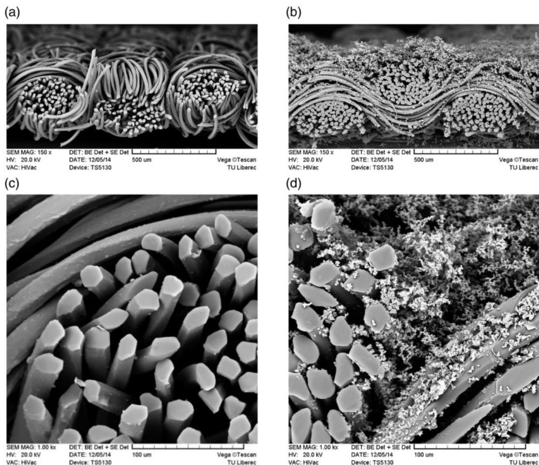
**Figure 11.** Cross section SEM pictures of PET/PPy textile composites prepared by following adjustments: (a),(c) 5°C, 1 h, 0.64 g/l, (b),(d) 15°C, 15 h, 5.8 g/l. Two different magnitudes were used: 150× and 1000×.
