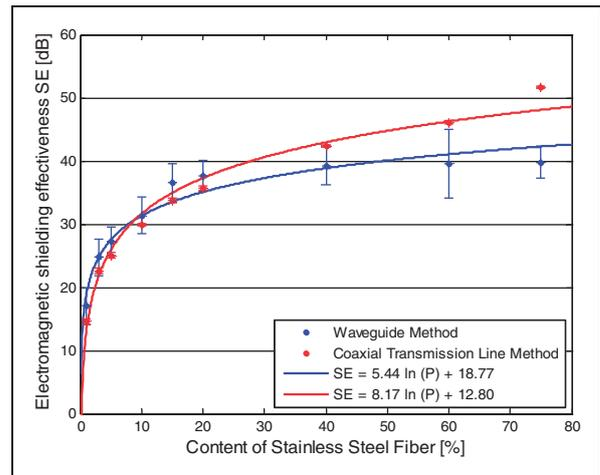
**Figure 7.** The dependence of electromagnetic shielding effectiveness at frequency 1800 MHz on metal fiber content for the whole sample set.
