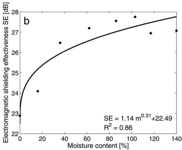
FIG. 10. The dependence of shielding effectiveness on moisture content of fabric at frequency (a) 1.5 GHz, (b) 2.45 GHz.
