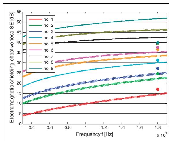
**Figure 5.** Frequency dependent electromagnetic shielding effectiveness measured by coaxial transmission line method (solid and dash line), points represent SE measured by waveguide method at frequency 1800 MHz.
