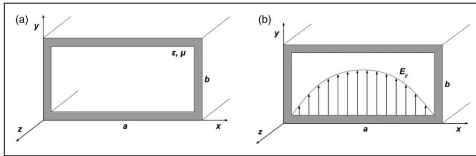
**Figure 2.** (a) Rectangular waveguide, (b) electric field inside the rectangular waveguide.
