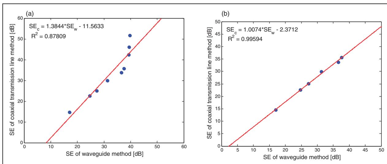
**Figure 8.** Quantile–quantile plot of SE data sets measured by the two measurement techniques (proposed waveguide method and comparative coaxial transmission line method) for (a) whole sample set, (b) sample set excluding samples with extremely high electrical conductivity.
