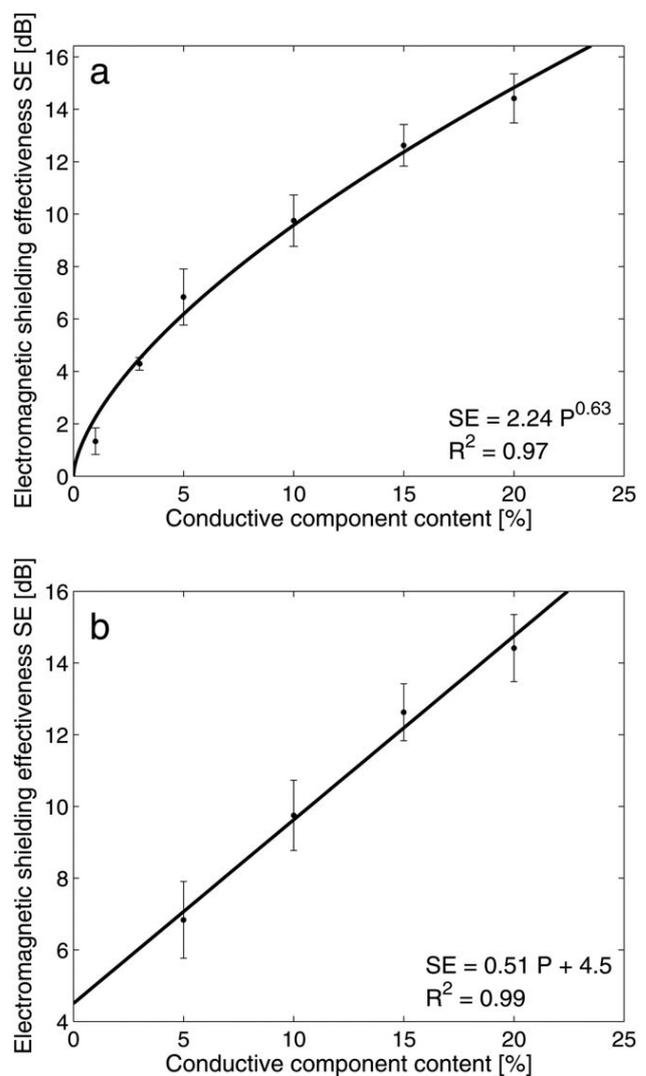
FIG. 7. The dependence of shielding effectiveness on metal fiber content for (a) samples: W1-5–W20-5, (b) samples with conductive component above percolation threshold: W5-5–W20-5.
