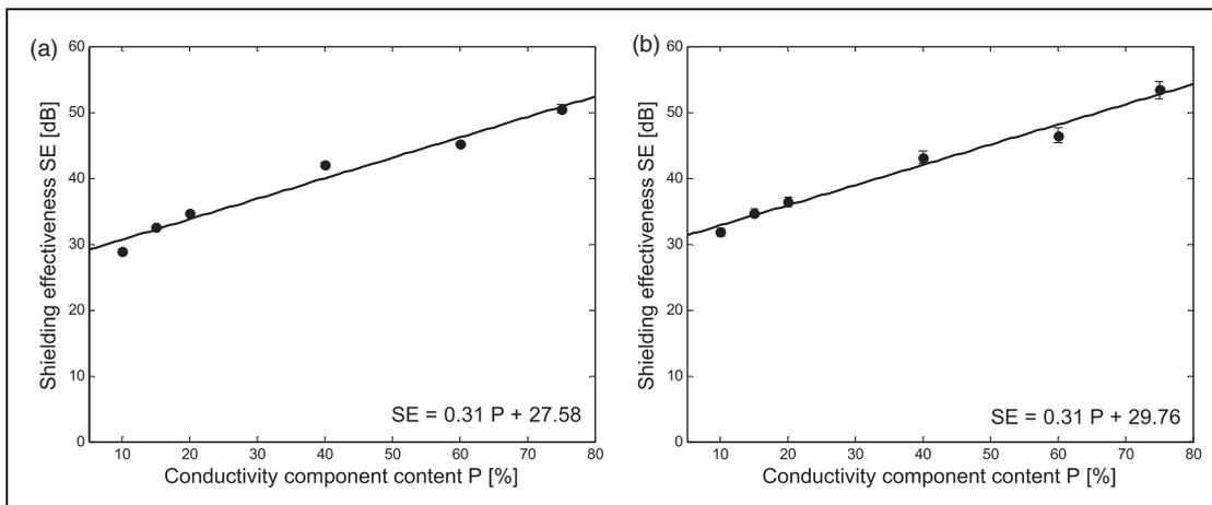
**Figure 5.** The dependence of shielding effectiveness on the conductivity component content for frequencies (a) 1500 MHz and (b) 2450 MHz.
