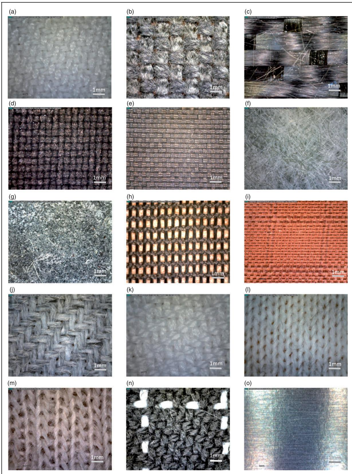
**Figure 1.** Microscopic images at 50 $\times$  magnification of samples: (a) "N Wo W"; (b) "Ca W 1"; (c) "Ca W 2"; (d) "PPy/PESW"; (e) "Mf Ag W"; (f) "Mf 20Eu NW"; (g) "Mc Al NW"; (h) "Mc Ag K"; (i) "Mc Cu/Ag W"; (j) "H 20SS W"; (k) "H ISS Ws1"; (l) "H 1SS Ks/j"; (m) "H 10SS Kd/j"; (n) "H 10SS WG"; (o) "F Al".
