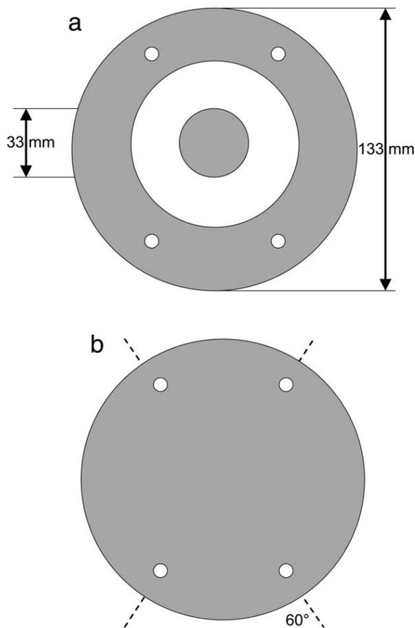
FIG. 4. Illustrations of (a) reference and (b) load sample.
