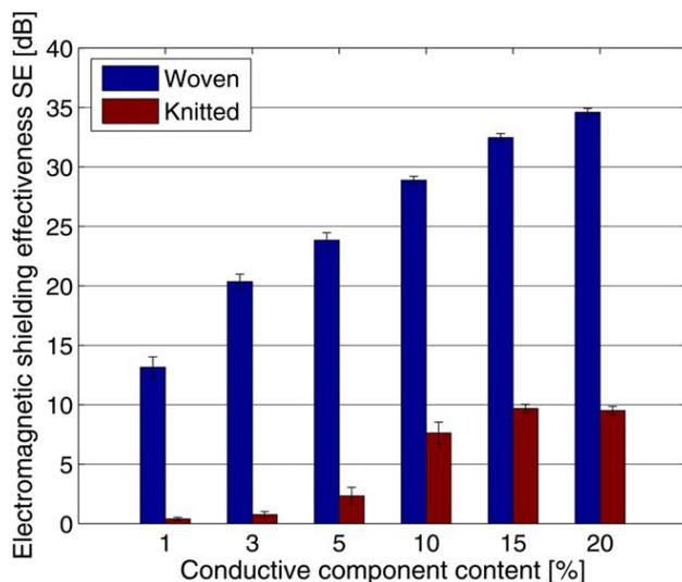
FIG. 13. Comparison of SE of samples with different structure (woven, knitted) at 1.5 GHz. [Color figure can be viewed at wileyonlinelibrary.com.]
