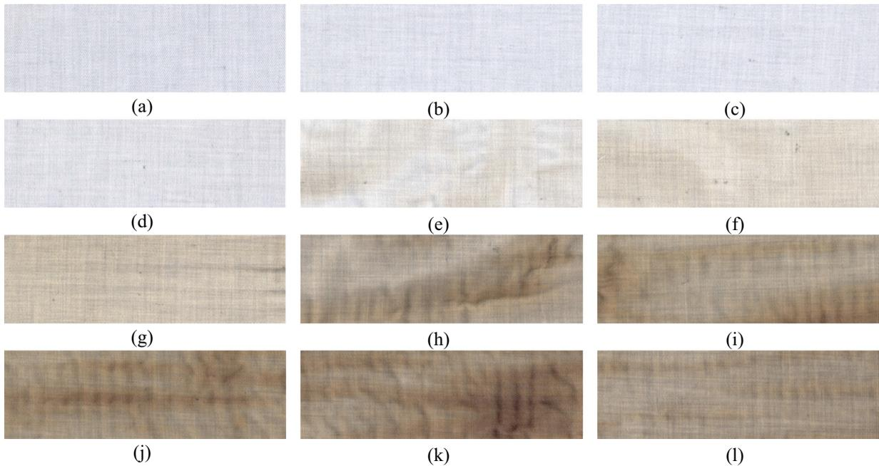
**Fig. 5.** Scanned images of samples irradiated by different intensity expressed by gray scale [%]: (a) 0%, (b) 7.5%, (c) 14.9%, (d) 19.2%, (e) 24.3%, (f) 27.8%, (g) 34.5%, (h) 39.2%, (i) 42.7%, (j) 46.7%, (k) 51.0, (l) 56.9%.
