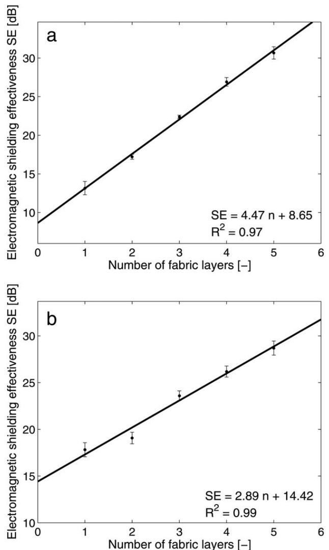
FIG. 9. The dependence of shielding effectiveness on number of fabric layers for frequency (a) 1.5 GHz, (b) 2.45 GHz.
