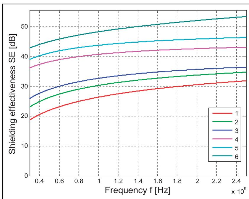
Figure 4. The dependence of measured electromagnetic shielding effectiveness on frequency for all samples.
