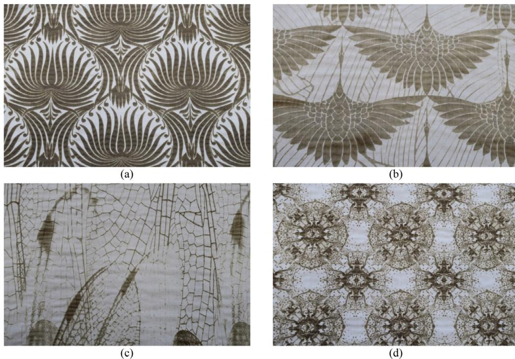
Fig. 11. Laser engraved functional (electrically conductive) samples: (a) pattern A, (b) pattern B, (c) pattern C, (d) pattern D.
