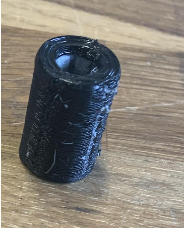
Figure 50: Linear Bearing - without Ooze Shield
