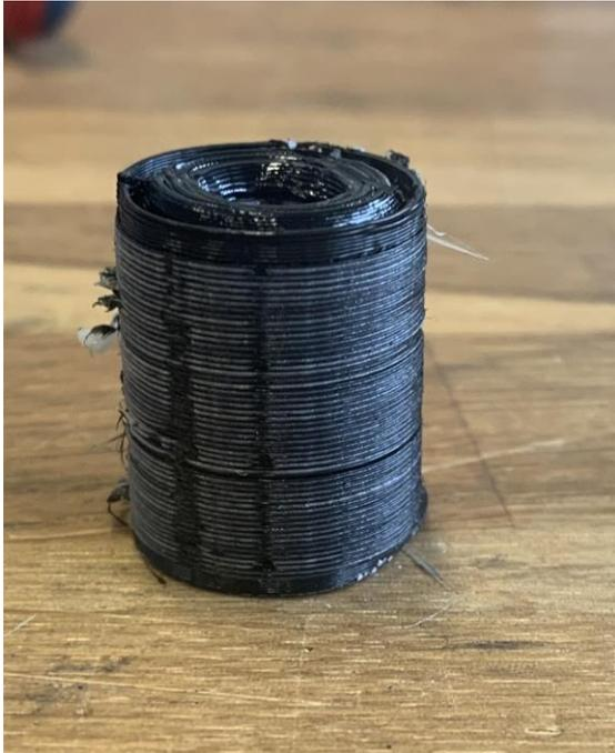
Figure 48: Linear Bearing – with Ooze shield
