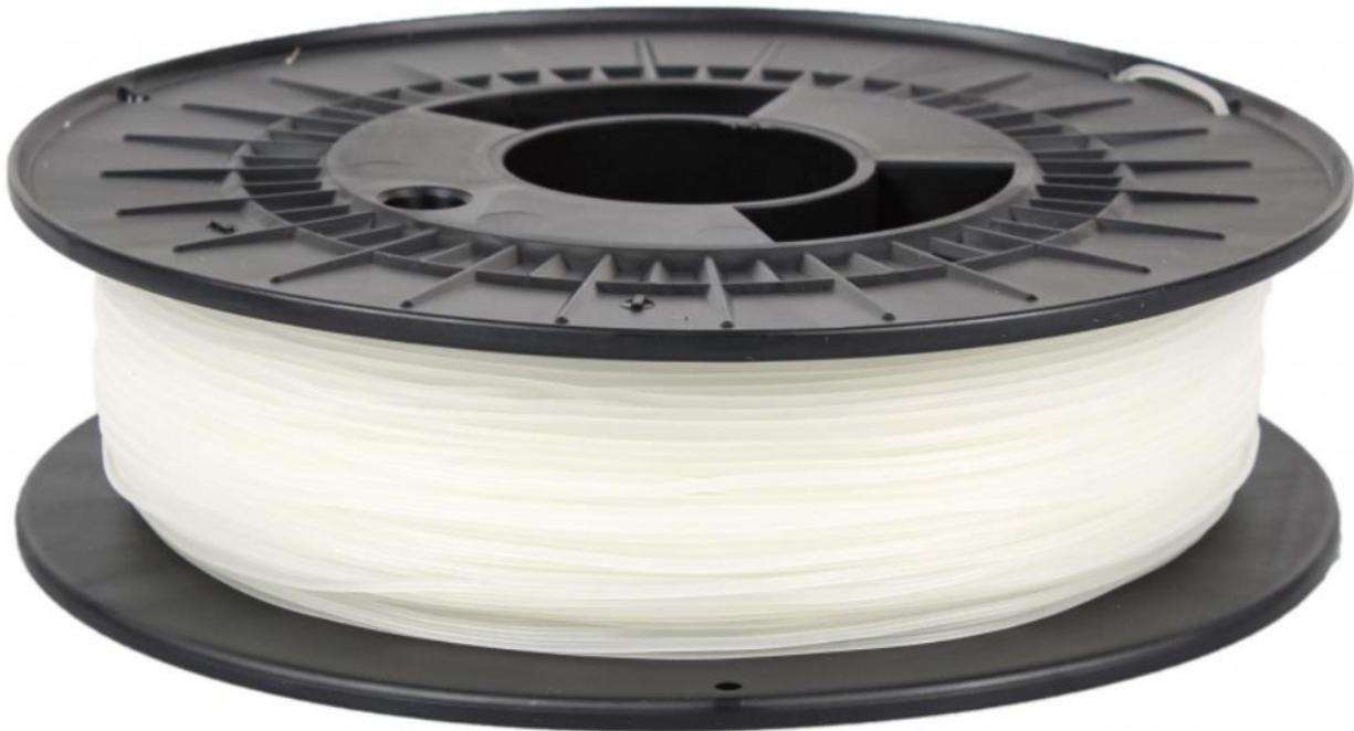
Figure 21: Filament of TPE 88 RubberJet [13]
