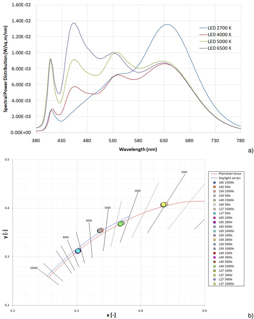
Figure 2 SPD of four LEDs (a) and position of light sources in CIE xy diagram at different conditions (b)
