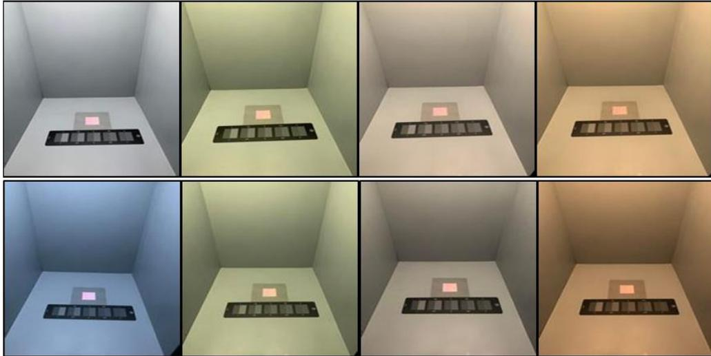
**Figure 3** Position of a sample pair and the grey scale in the viewing cabinet at maximum (top) and minimum (bottom) luminance levels
