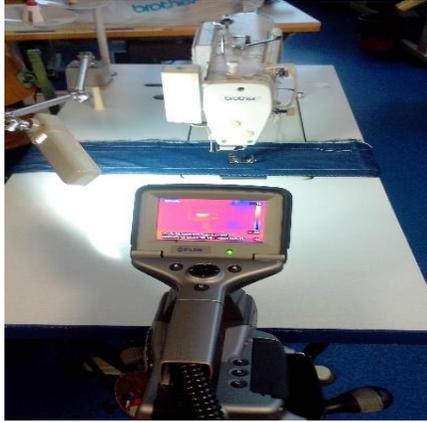
Figure 8 Thermal camera FLIR P60 with Lockstitch machine
