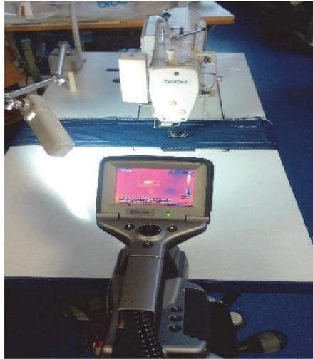
Figure 1. Thermal camera FLIR P60 with Lockstitch machine
