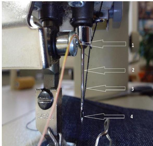
**Figure 13 Placement of the thermocouple**
