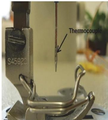
Figure 10. Inserted thermocouple
