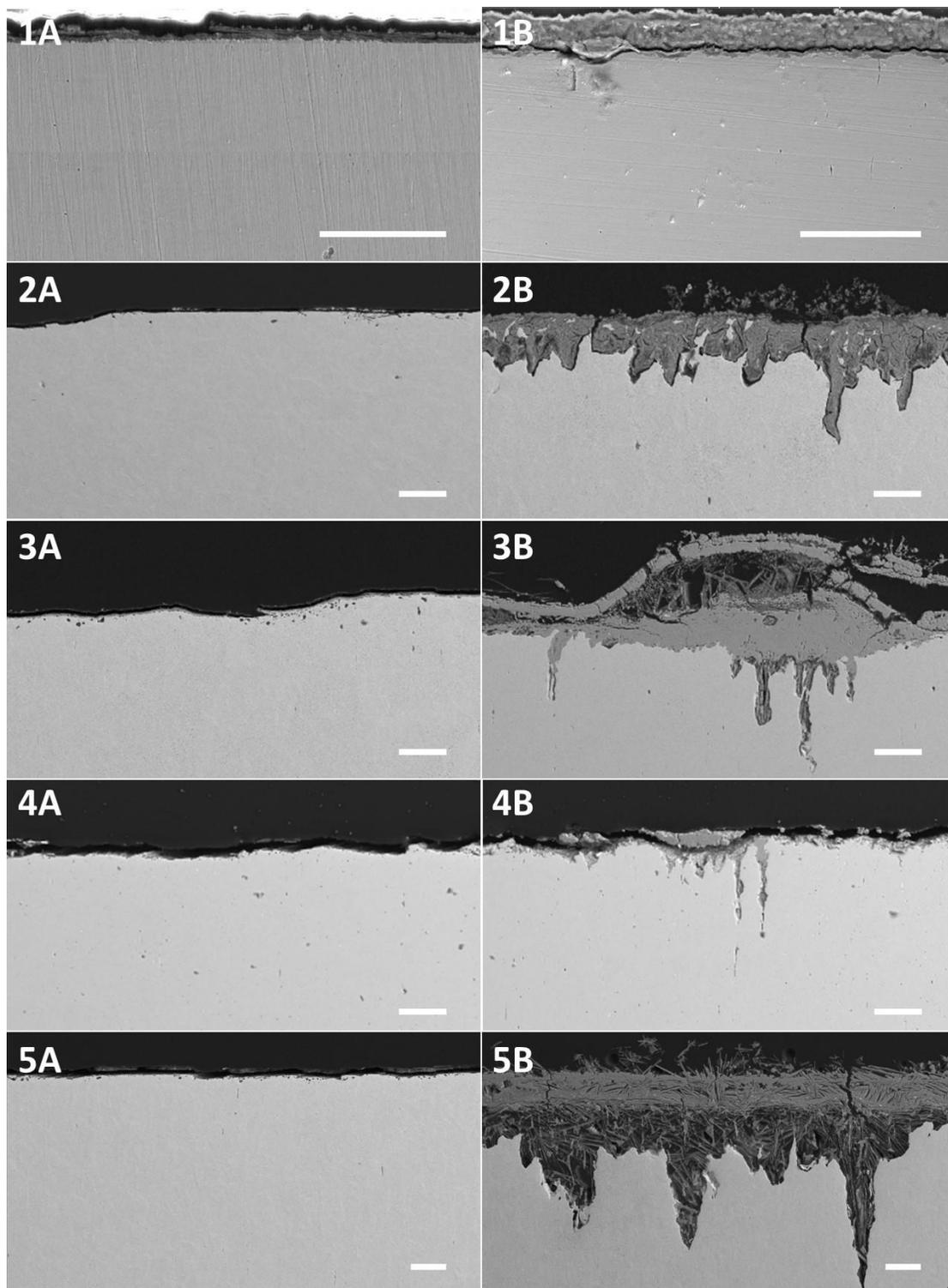
Figure 50: SEM micrograph presenting MIC – a cross-section of the carbon steel A belongs to abiotic (left) and B belongs to biotic samples (right) where the numbers 1, 2, 3, 4, and 5 represents sampling time after 3, 6, 12, 18 and 26 months, respectively. The scale bar used for each image was 50  $\mu\text{m}$ .
