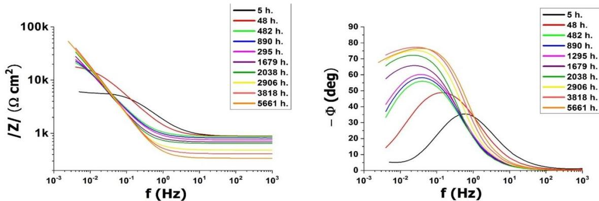
*Figure 34: Bode plots of electrochemical impedance spectra time evolution for carbon steel under sterile conditions.*
