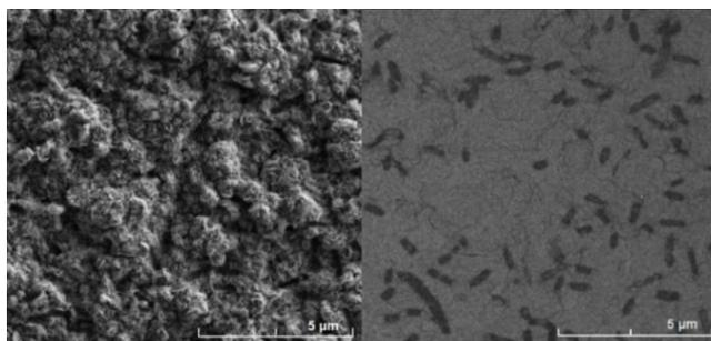
*Figure 39: Scanning electron micrograph of the biofilm formed on carbon steel exposed under non-sterile conditions after 240 days incubation – comparison of different detector modes (left SE detector, right In-Beam BSE detector).*
