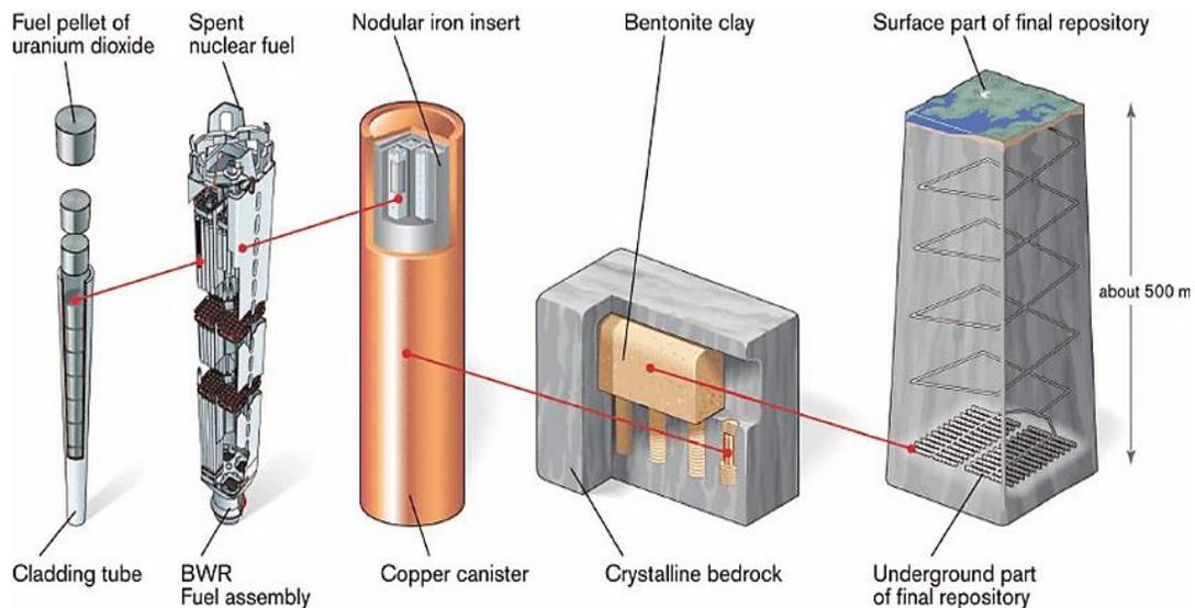
Figure 4: The KBS-3 concept for disposal of spent nuclear fuel by Svensk Kärnbränslehantering AB (SKB) (AB, 2011).
