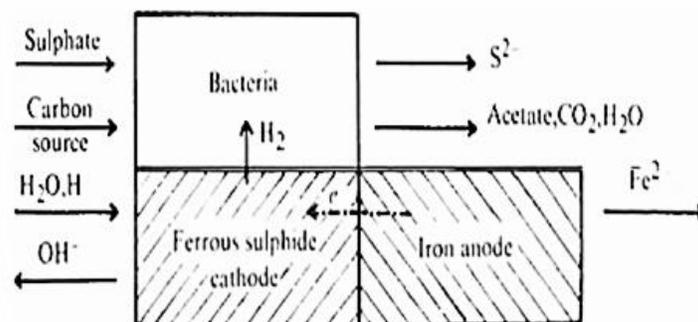
Figure 15: Corrosion of metal by SRB proposed by King's Mechanism (King and Miller, 1971).
