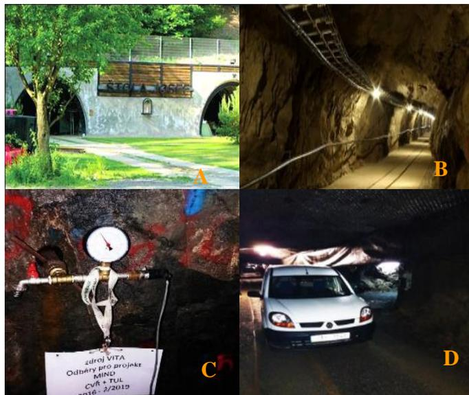
Figure 22: Images representing Josef URC. A) Entrance to Josef URC B) Underground tunnel C) Main tap of source VITA water under 2.5 bar and D) Transport of VITA water in the Josef URC tunnel.
