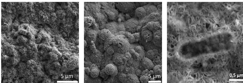
*Figure 38: Scanning electron micrographs showing the surface of carbon steel covered by a thick layer of spherical or rod-shaped microorganisms (SE detector).*
