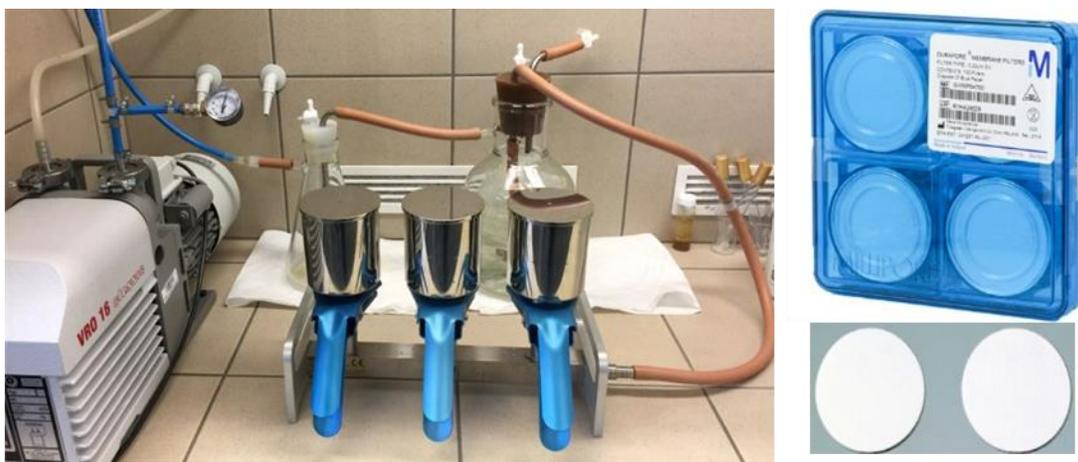
Figure 24: Filter apparatus for filtration of water (left), 0.22 µm GV Durapore® filter membrane (right).
