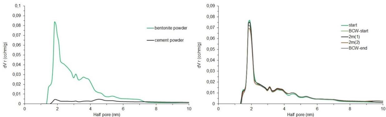
Figure 65: Pore size distribution evaluated by DFT method. On the left - comparison of the pure bentonite and concrete powder. On the right - comparison of the concrete containing samples at the beginning (start and BCW-start) and the end of the experiment (2m, BCW-end). Start and 2m – bentonite concrete samples, BCW – control samples (bentonite, concrete, sterile water).
