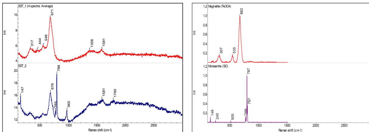
Figure 52: Raman spectra of carbon steel in SBPOW under sterile anaerobic conditions after 26 months denoting magnetite and silicon carbide (SiC) (left) and Standard spectra from the RRUFF library (right) (Lafuente et al., 2016).
