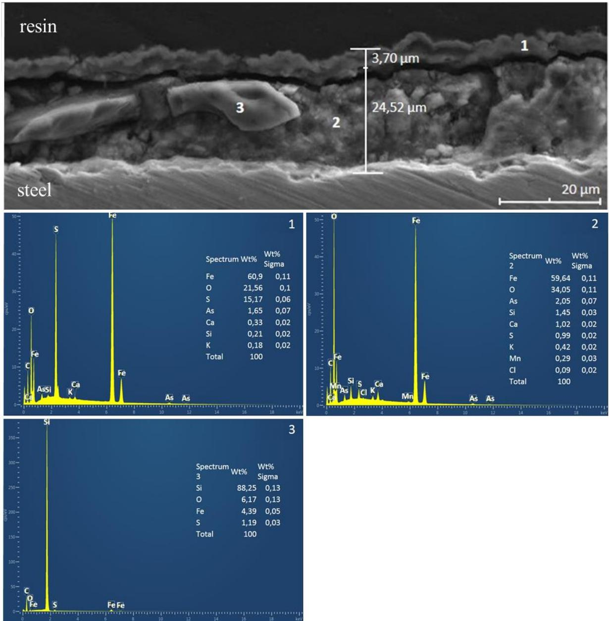
Figure 42: Scanning electron micrograph showing the formation of a corrosion layer. The image shows a sample cross-section with bacteria present (above) and the respective X-ray spectra of positions 1, 2, and 3 (below).
