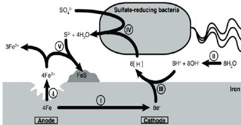
Figure 14: Scheme of iron surface corrosion induced by SRB based on the process postulated by the cathodic depolarization theory following 5 major steps starting with the dissolution of iron (I), dissociation of water (II), proton reduction (III), sulfate reduction (IV) and finally, sulfide precipitation (V) (Mori et al., 2010).
