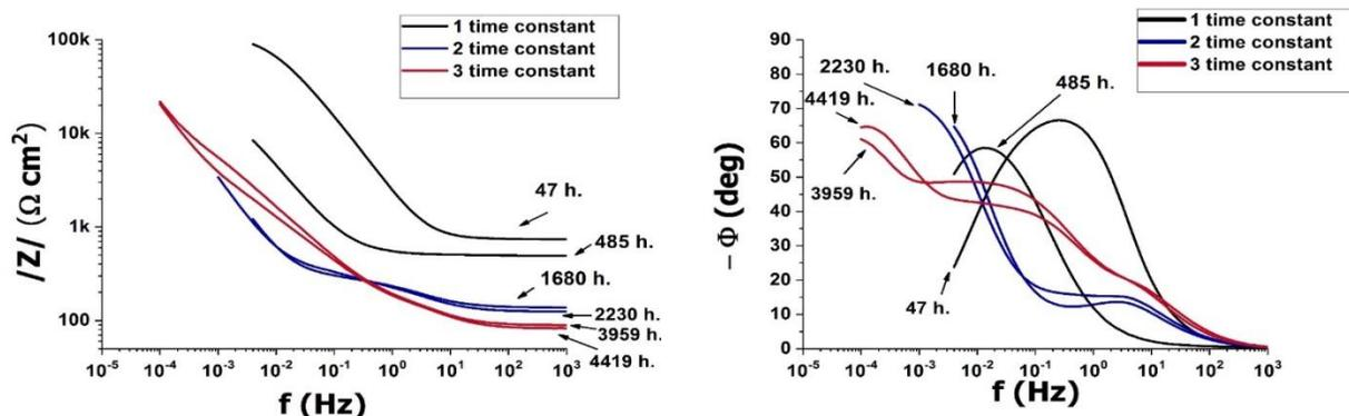
Figure 35: Bode plot of electrochemical impedance spectra time evolution for carbon steel under non-sterile conditions.
