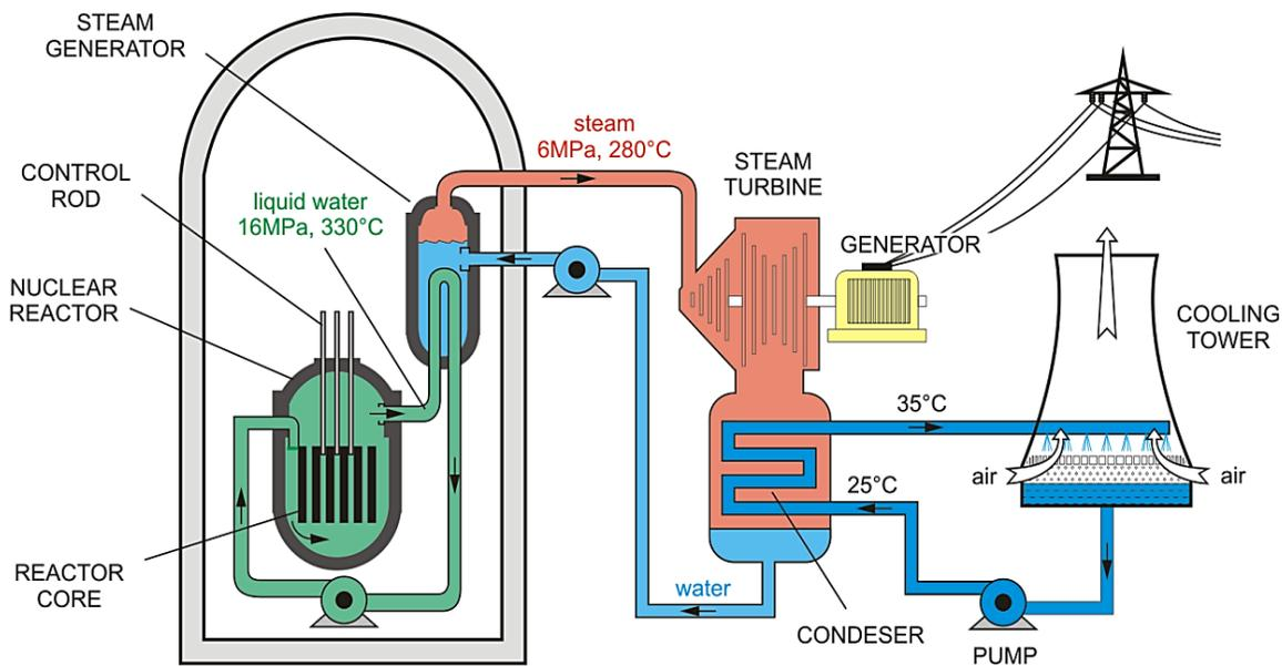
*Figure 1: Diagram of Nuclear energy power plant.*
