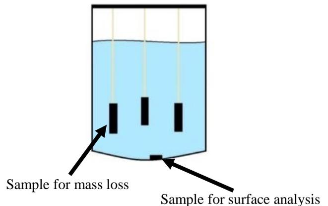
*Figure 47: Experimental design for corrosion in SBPOW.*
