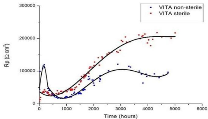
Figure 37: Time evolution of polarization resistance.
