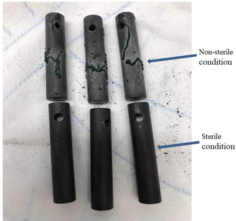
*Figure 51: Test specimens of the carbon steel under non-sterile and sterile conditions collected after 26 months. Black turbidity was observed on the surface of the testing coupon. A clear sign of corrosion is seen on the surface of carbon steel under the biotic environment.*
