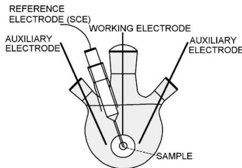
*Figure 33: Experimental corrosion cell.*
