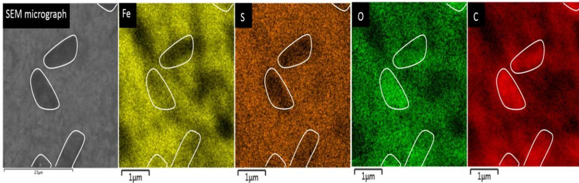
*Figure 40: Energy-dispersive X-ray elemental maps of the corroded region with bacteria present (marked with a white line).*
