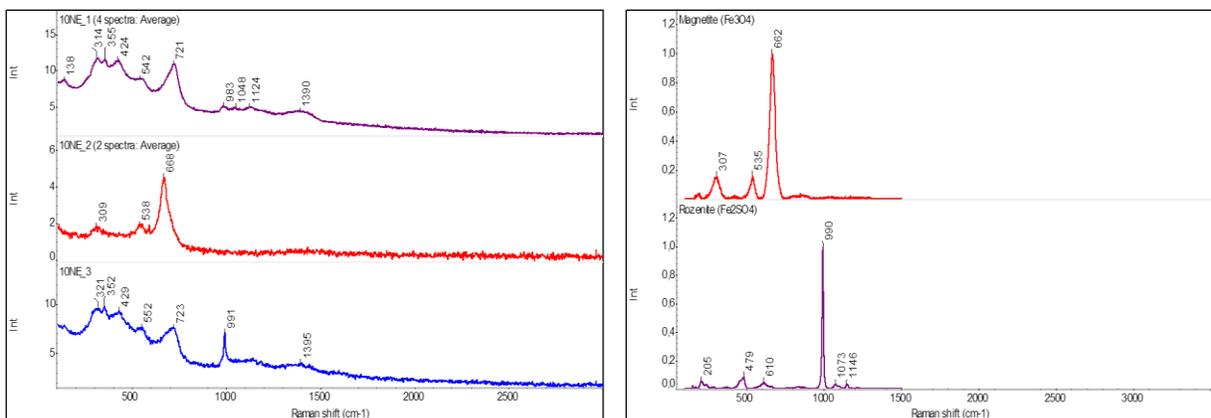
Figure 53: Raman spectra of carbon steel in SBPOW under non-sterile anaerobic conditions after 26 months of indicating the presence of akaganeite, magnetite, and rozenite (left) and standard spectra from the RRUFF library (right) (Lafuente et al., 2016).
