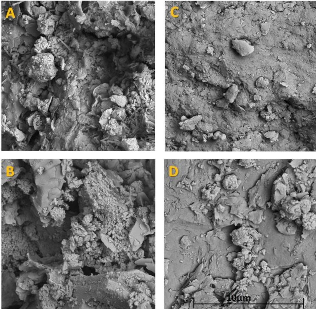
*Figure 64: SEM micrograph of the samples: A) bentonite concrete sample (bentonite, concrete and VITA water) start, B) bentonite concrete sample end (2m), C) BCW (bentonite, concrete and sterile water) start, D) BCW end (2m). The scale bar used for each image was 10  $\mu$ m.*
