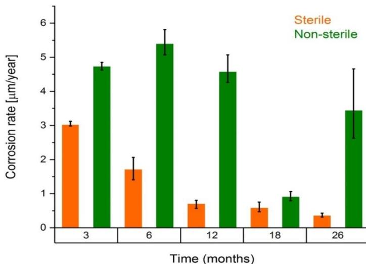
Figure 48: Average corrosion rates based on weight loss measurements for the carbon steel in a sterile environment (orange) and in the environment enriched with microorganisms (green).
