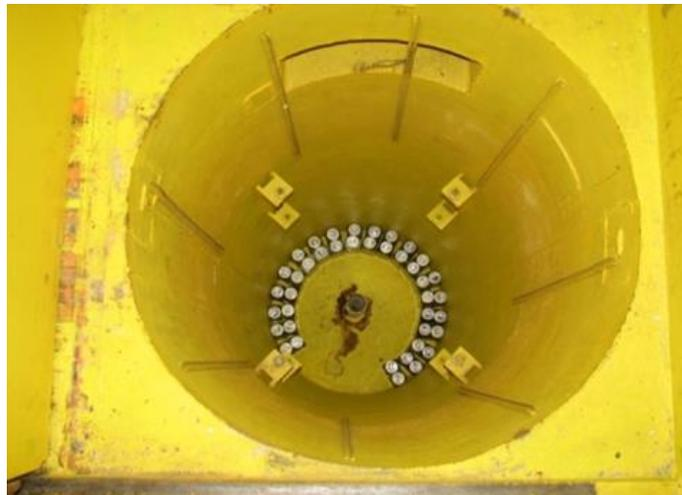
*Figure 26: Samples inside the irradiation chamber, diameter about 100 cm.*
