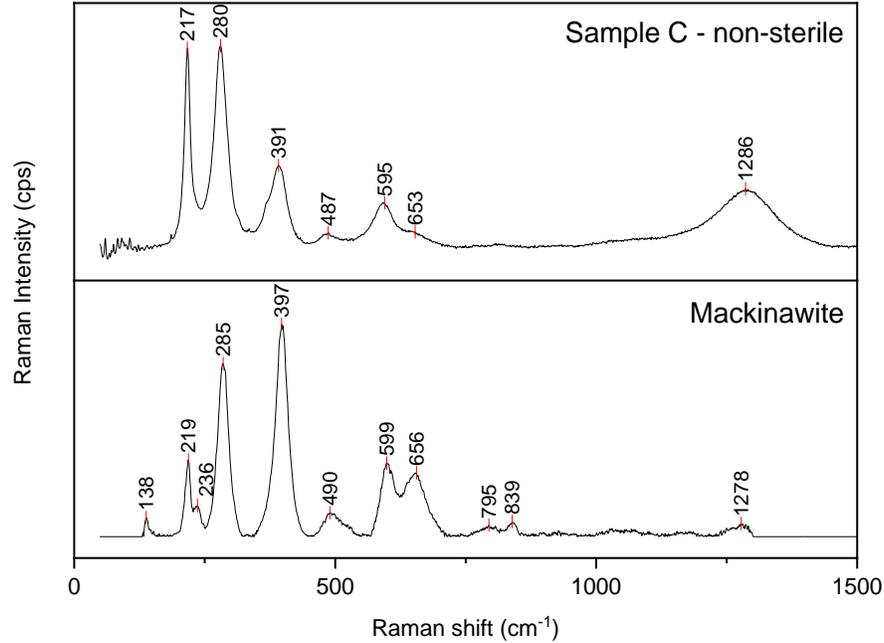
Figure 44: Raman spectra of carbon steel under non-sterile anaerobic conditions in VITA water after 293 days (top) and mackinawite standard (bottom).
