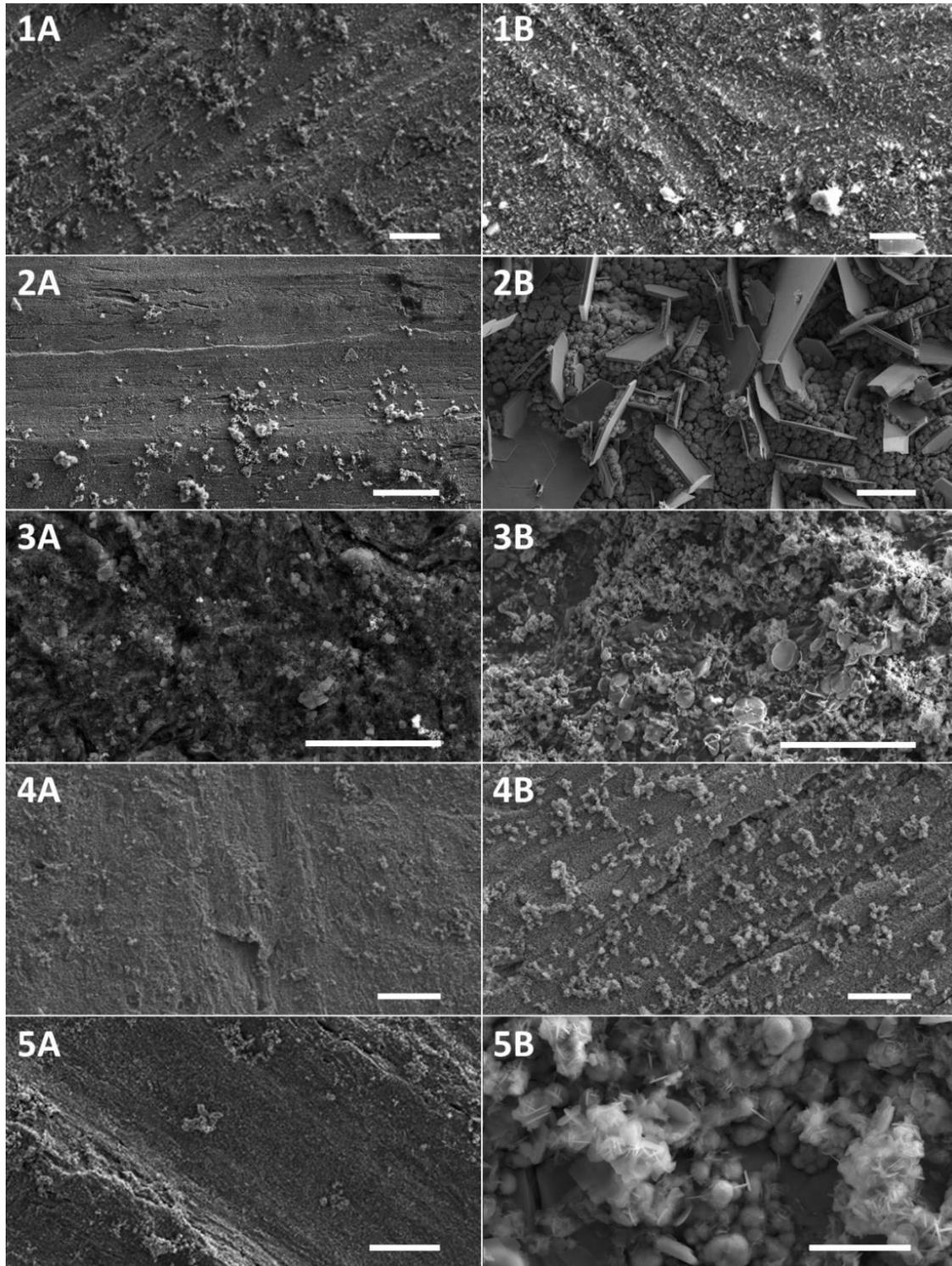
*Figure 49: SEM micrograph presenting the surface of carbon steel. A belongs to abiotic (left) and B belongs to biotic samples (right) where the numbers 1, 2, 3, 4, and 5 represents sampling time after 3, 6, 12, 18, and 26 months, respectively. The scale bar used for each image was 20  $\mu\text{m}$ .*
