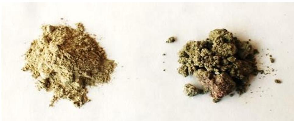
*Figure 23: Homogenized bentonite on the left and raw (unhomogenized) bentonite on the right.*
