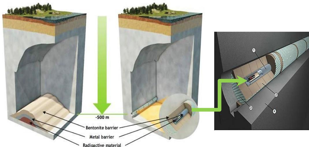
*Figure 5: Concept of geological disposal of High level and long-lived waste (Left) and a super container in a disposal borehole where number 1 represents a container, 2– pre-cast bentonite elements, 3- external basket from perforated steel sheet and 4– host rock (Right) (SÚRAO 2016).*
