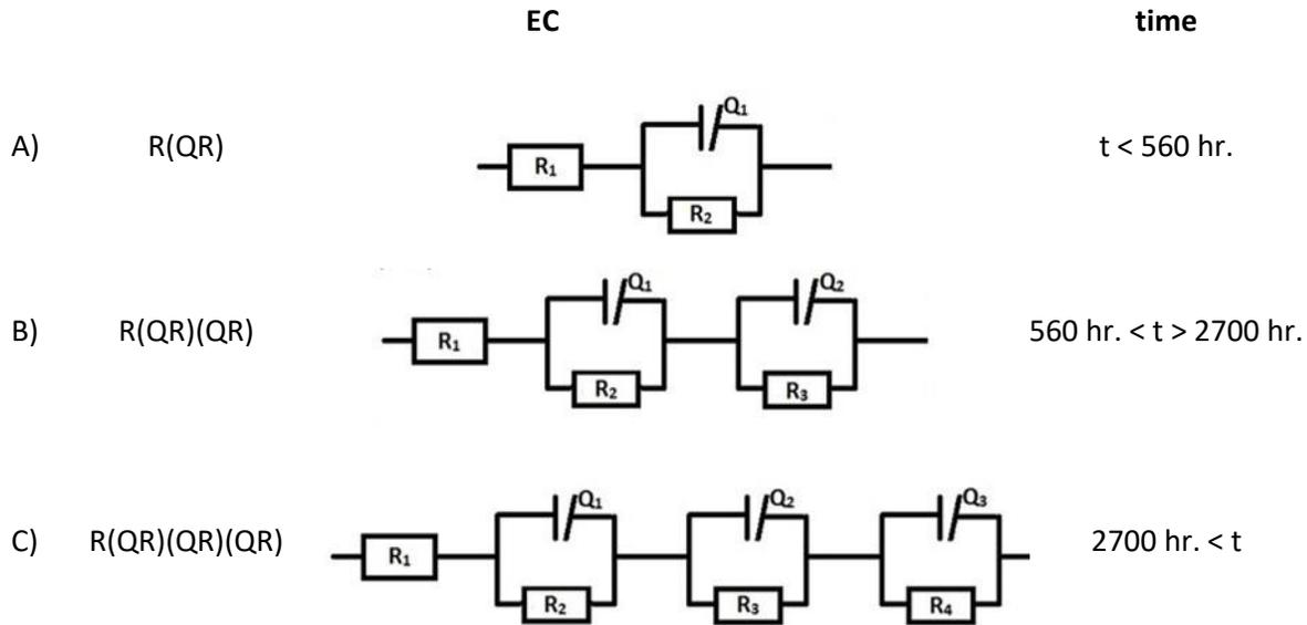
Figure 36: Equivalence circuits used for electrochemical impedance spectroscopy data fitting and time evolution of corrosion stages.
