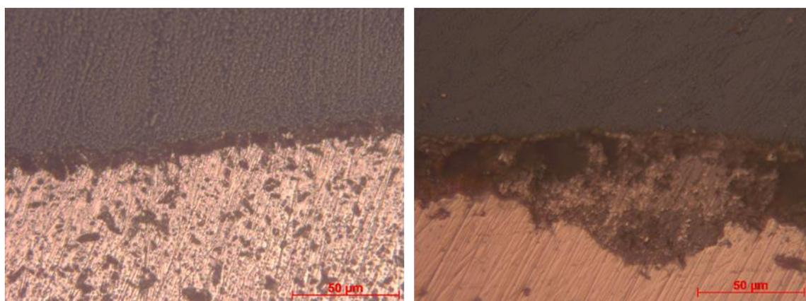
*Figure 43: Cross-sections of the sterile (left) and non-sterile (right) steel after exposure.*
