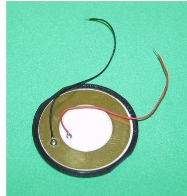
Fig.2.2 Piezoceramic transducer
