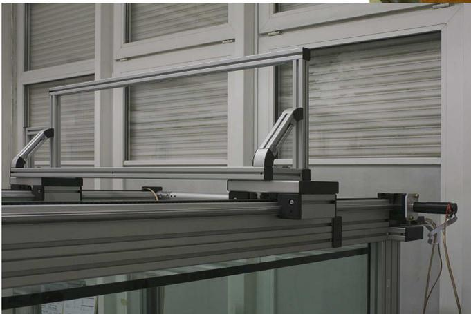
Detailed view on traverse system with motor
