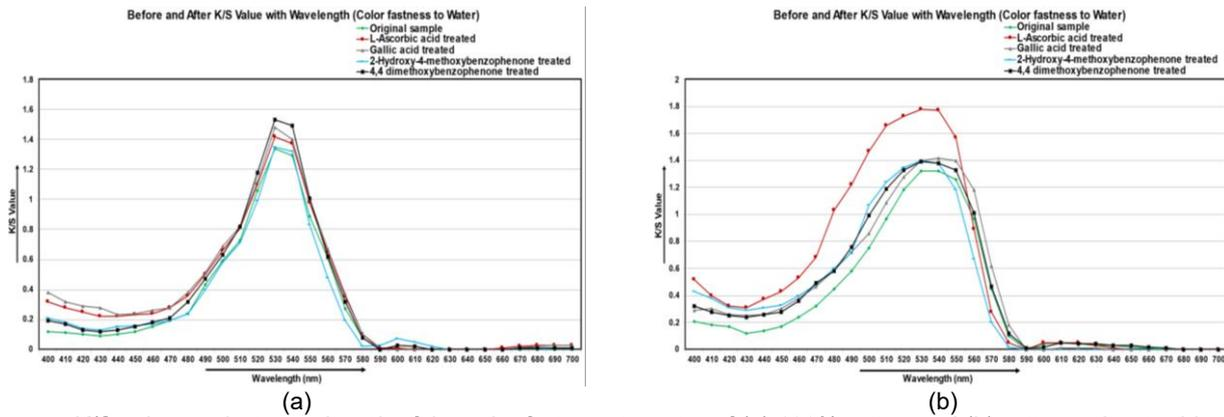
**Figure 4** K/S value against wavelength of the color fastness to water of (a) 100% cotton and (b) cotton-polyester blended fabric
