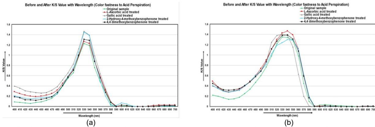
**Figure 5** K/S value against wavelength of the color fastness to acid perspiration of (a) 100% cotton and (b) cotton-polyester blended fabric
