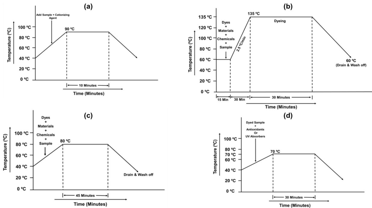
**Figure 2** Process Sequences of (a) cationization process (b) polyester dyeing (c) cotton dyeing (d) antioxidants and UV absorbers application
