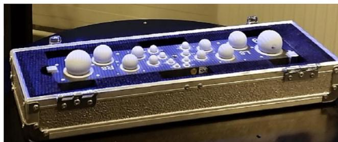
**Figure 2:Standard part of GOM for Calibration[5]**
