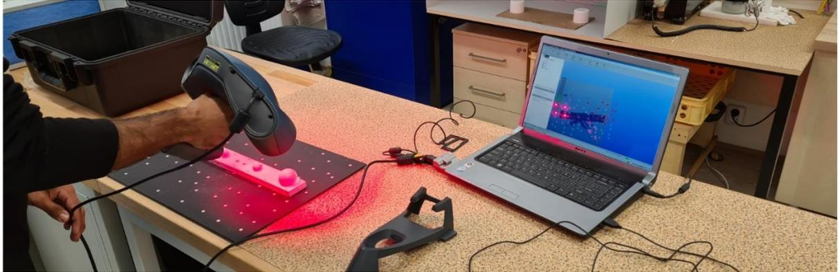
*Figure 46: Scanning with REV-scan*
