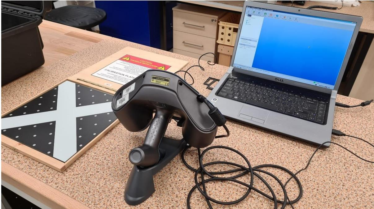
**Figure 45: REV-scan Calibration with Calibration plate in VX scan software**
