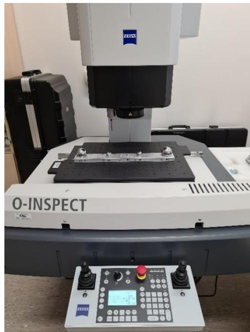
**Figure 22: Zeiss O-INSPECT 322 CMM**
