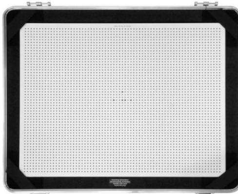
**Figure 30: Calibration Panel CP40 for MV320[22]**
