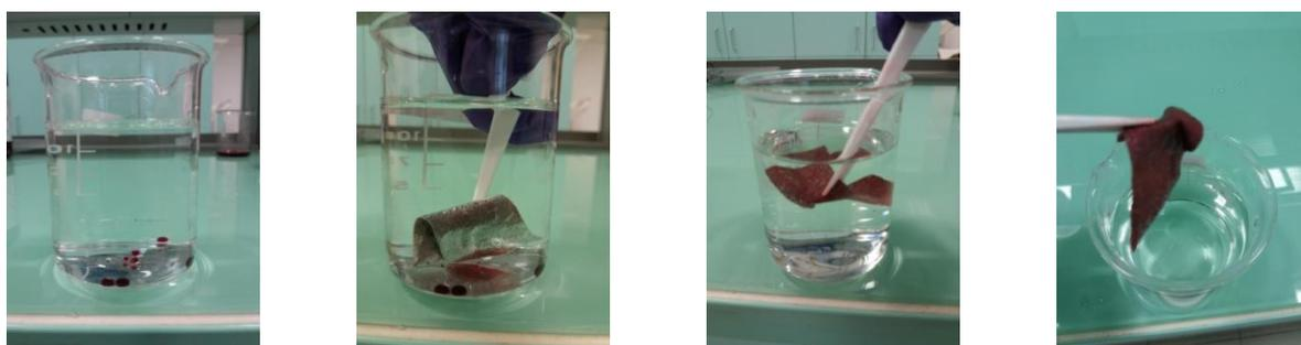
(b). Photographs of chloroform removal from underwater surface
