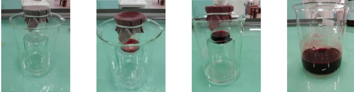
(c). Photographs of oil in water separation experiment
