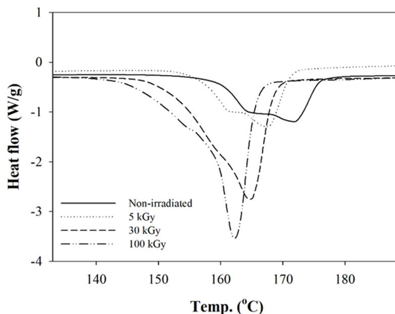
Figure 6. DSC thermogram exhibiting the  $T_m$  at different irradiation doses.
