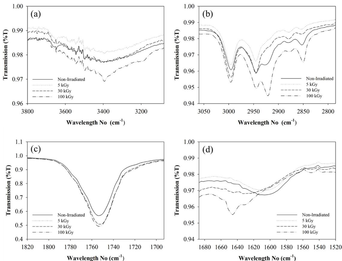
**Figure 4.** FTIR spectrum shows the chemical interaction in polymeric phase under different doses of electron-beam irradiation of (a) O–H bond, (b) C–H<sub>3</sub>, (c) C=O and (d) COO<sup>-</sup>.
