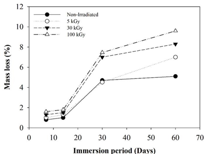
**Figure 13.** Mass loss of the PLLA/CMS/ $\beta$ -TCP exposed under different irradiation doses of electron beam after 60 days immersion in PBS medium.
