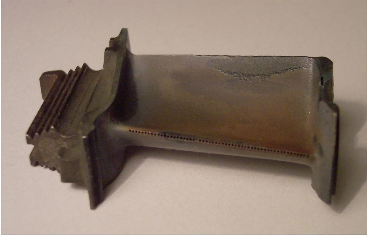
Figure 2.3: Cavitation Erosion on Blade
