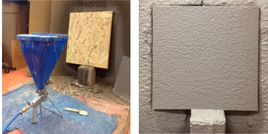
**Figure 29.** Images illustrating the process of spraying geopolymer mixture and representation of unmodified surface (OSB panel) in the left and coated surface by GF (right).
