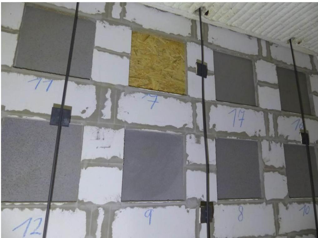
**Figure 92.** The samples inside furnace numbered from left to right in the 1<sup>st</sup> row (11, 7, 17, 16) and the 2<sup>nd</sup> row (12, 9, 8, 10).
