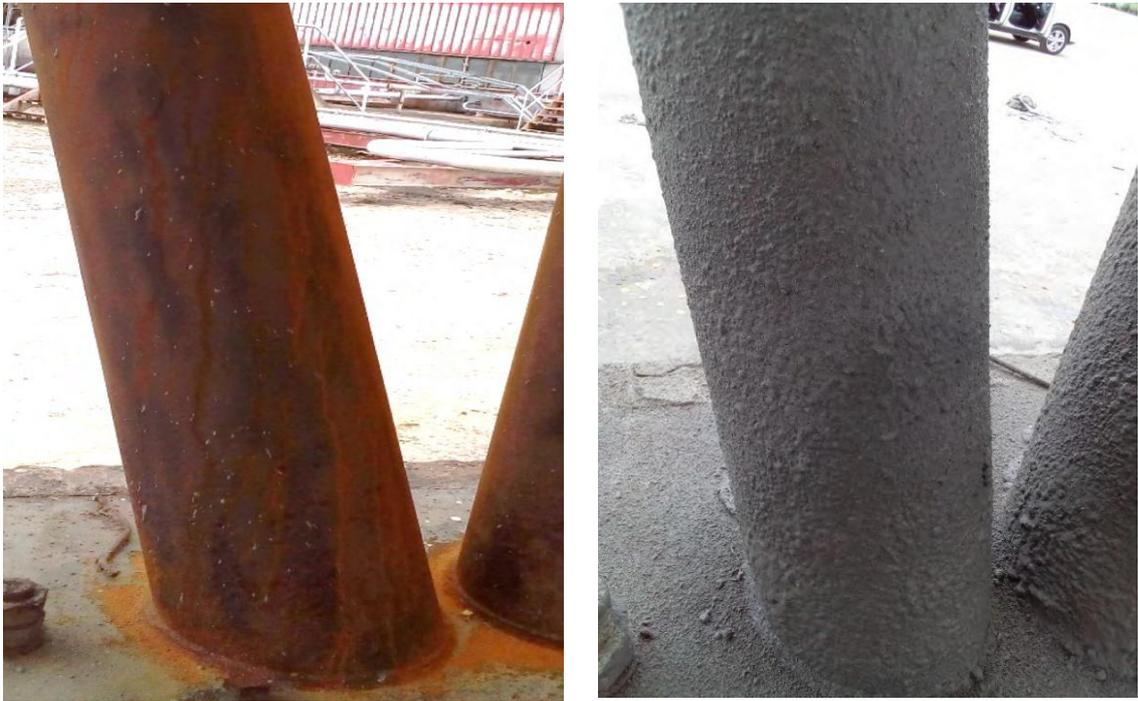
**Figure 127.** The surface of the pillars before (left) and after (right) spray-coating the GF layer.
