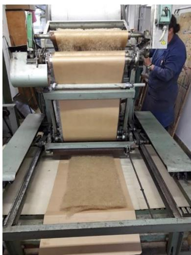
**Figure 1.** Production of a flax fibre mat.
