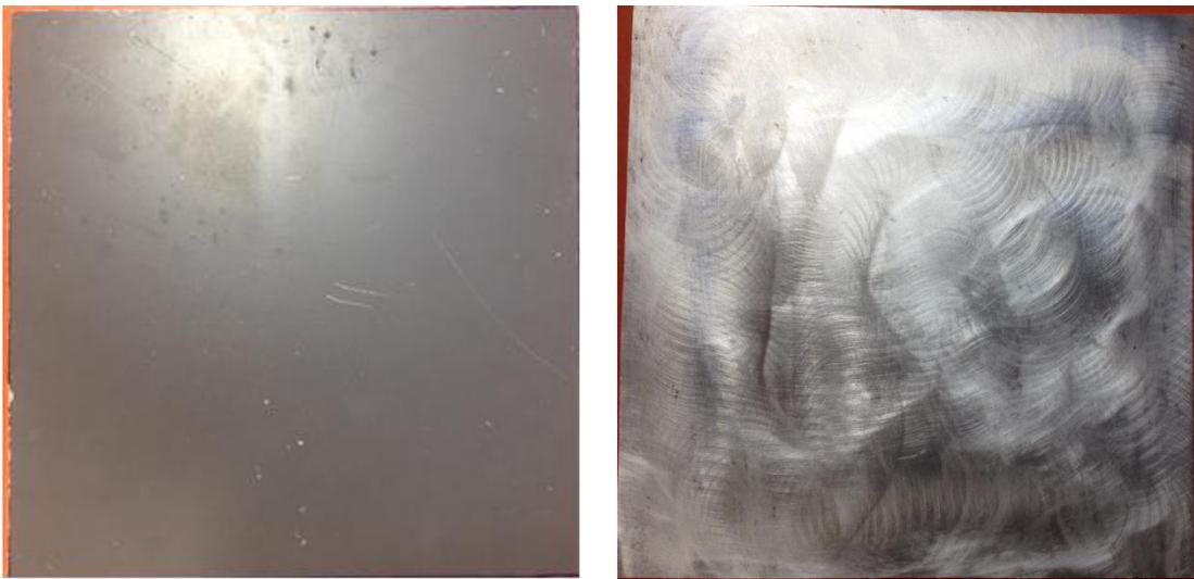
**Figure 63.** Both surfaces of an aluminum plate: original (left) and grinding (right).
