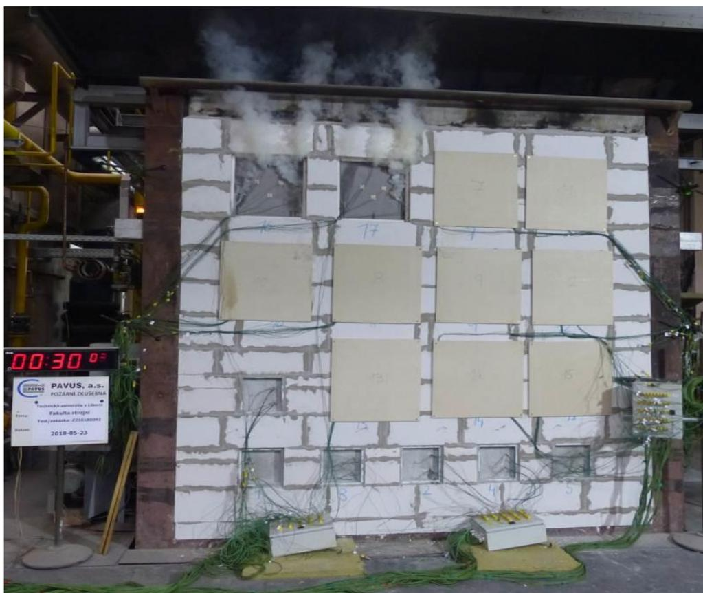
**Figure 94.** The view from outside after 30 min testing.
