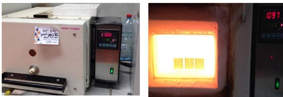
**Figure 33.** Furnace BINDER (left) and GFs in the furnace at 1100 °C (right).
