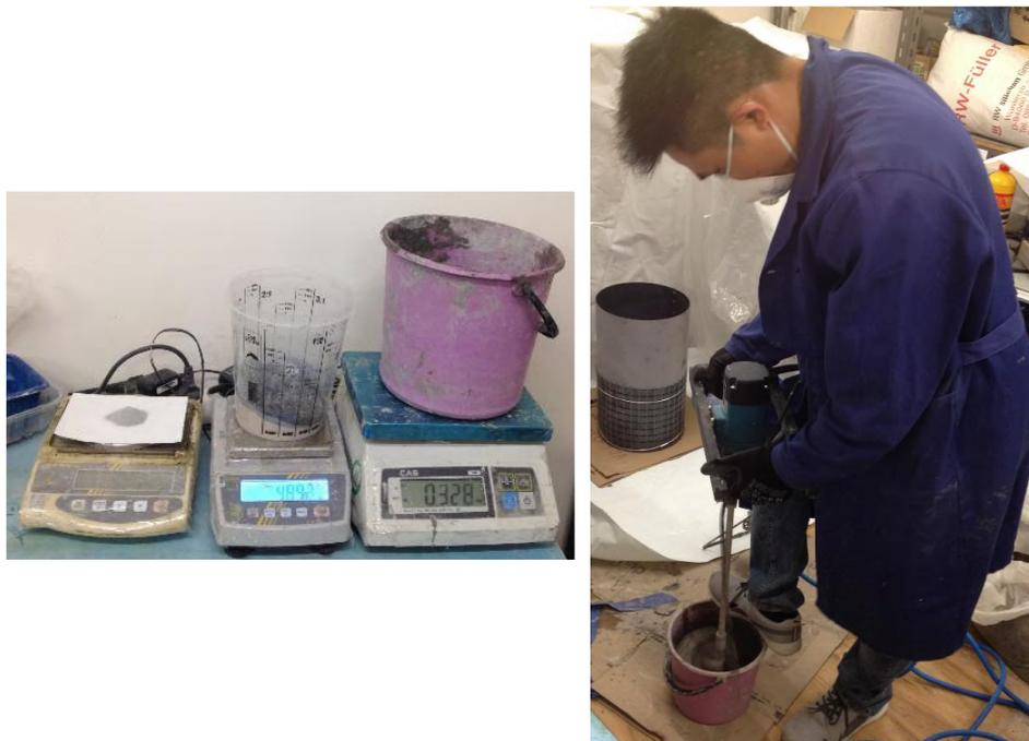
**Figure 72.** Preparing constituent materials (left) and mixing mortar for spraying (right).
