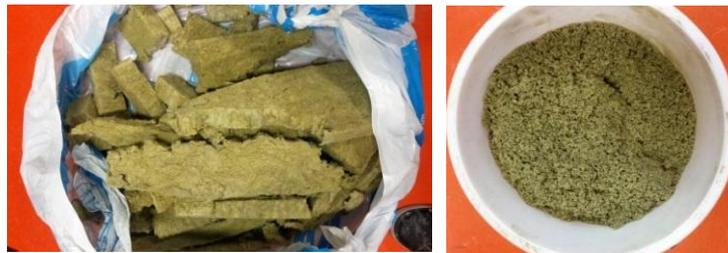
**Figure 34.** The photographs showing original basalt waste fibers (left) and modified basalt waste fibers after grinding (right).
