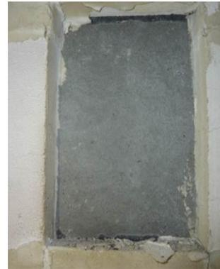
Sample 3, protection thickness 20.6 mm
