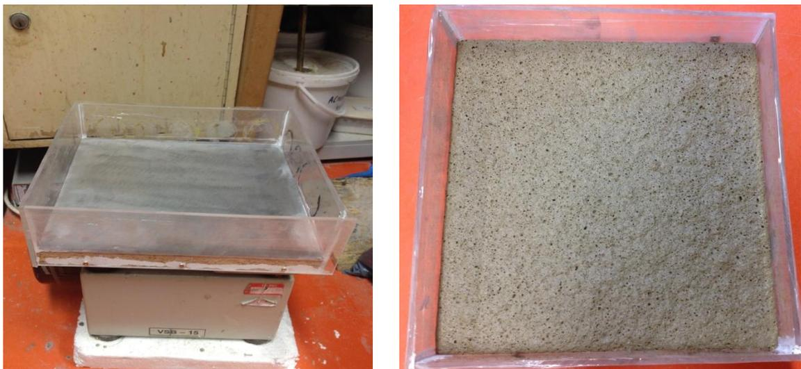
**Figure 64.** Preparation of geopolymer mixture and its application on the surface of Al plates.
