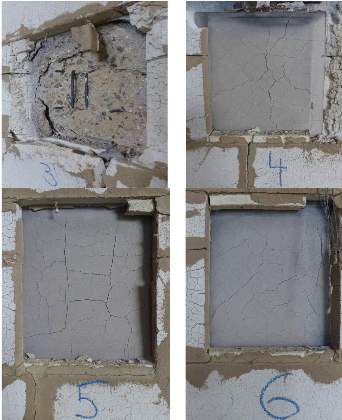
**Figure 97.** Detail of samples 3 to 6 with different protection thicknesses.
