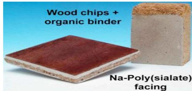
**Figure 12.** The fire-resistant wood-chipboards manufactured from geopolymer (na-poly(sialate)) [31].
