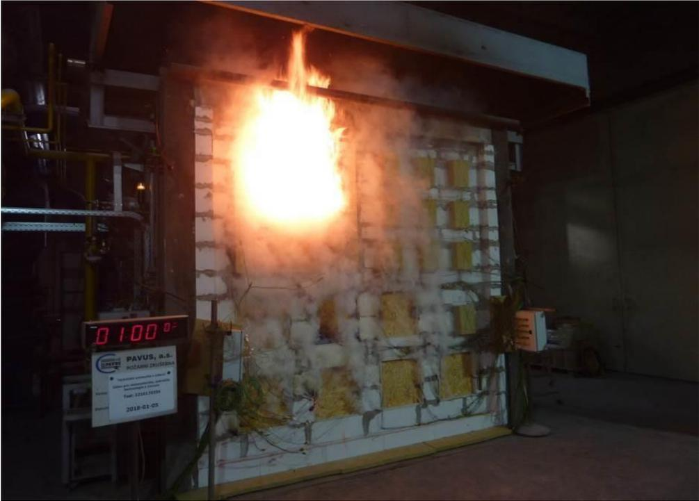
Figure 122. The sample after 60 min testing. The view from outside.
