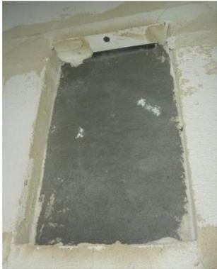
Sample 6, protection thickness 11.4 mm
