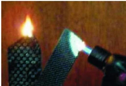
**Figure 19.** A carbon-epoxy aerospace composite (left) is burning while a carbon-geopolymer composite (right) still resists a 1200 °C fire [31].
