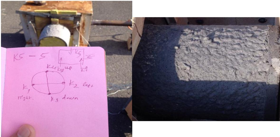
**Figure 75.** The position of thermocouples (left) and an outer image after testing (right).
