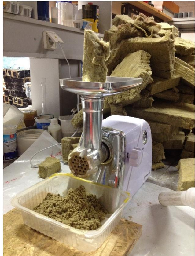
**Figure 2:** Photograph of basalt fibre grounded using the mill.
