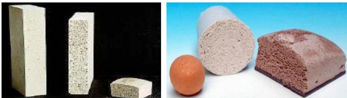
**Figure 16.** Example of foamed geopolymer materials [31].
