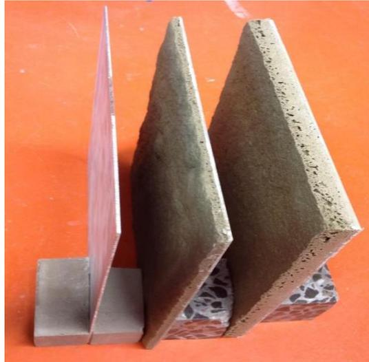
**Figure 65.** A photograph showing uncoated Al plate (left) and coated Al plates with 10 mm thickness of GF layer (middle) and 20 mm thickness of GF layer (right).
