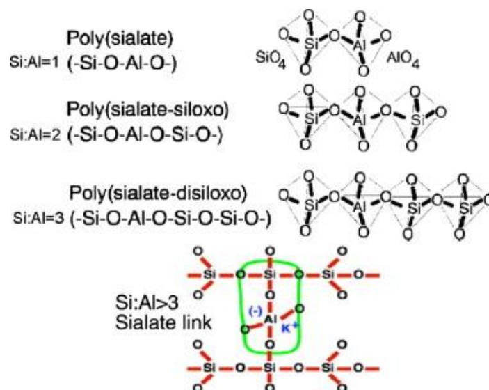
**Figure 21.** The structure of the geopolymer consists of a polymeric Si - O - Al chain [45].
