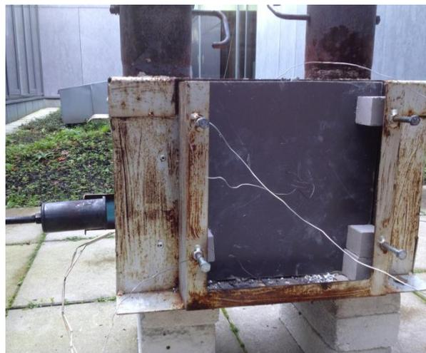
**Figure 66.** An image showing the sample layout on the test furnace.
