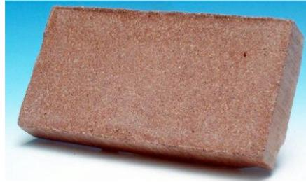
**Figure 14.** The geopolymer composite brick L.T.G.S. [31].
