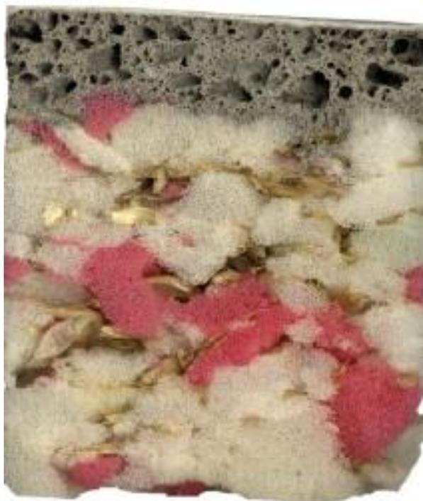
**Figure 137.** View of sandwich panel cut.
