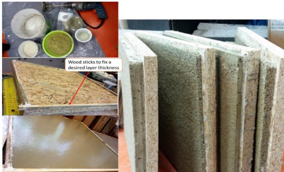
**Figure 36.** Materials and sample preparation steps to create a GF layer on the surface of the OSB panels.
