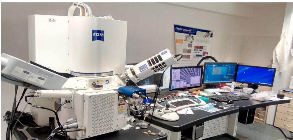
**Figure 31.** Carl Zeiss Ultra Plus SEM with Oxford micro-analytical system.
