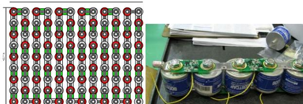
**Figure 8-** 650 Farad U-cap, 108 cell series string
