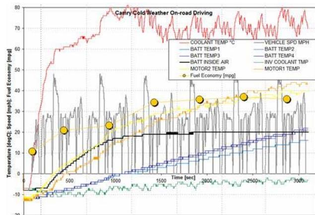
**Figure 7-** Cold Weather operation ( $-12^{\circ}\text{C}$ ) of an HEV Camry, with air cooled NiMH battery pack
