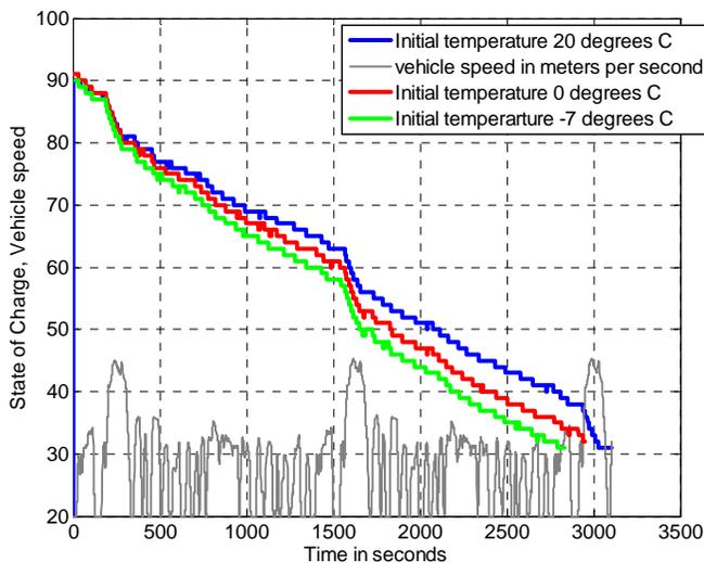
Fig 3. Drop in state of charge for the three initial temperatures over consecutive urban cycles.
