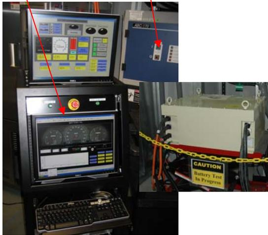
Fig 2 Battery HIL control and data acquisition rack, and high voltage DC power supply JCS VL41M with coolant, power and control connections
