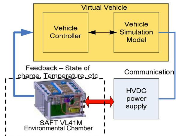
Fig 1. Block diagram of the Battery HIL test
