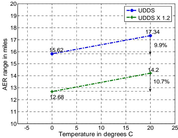
Fig 6: AER comparison between UDDS and UDDS X1.2 for 20°C, 0°C
