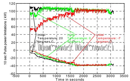
Fig 4. Propulsion and regen pulse power restrictions (red; -7°C initial temp., green; 0°C initial temp., black; 20°C initial temp.).
