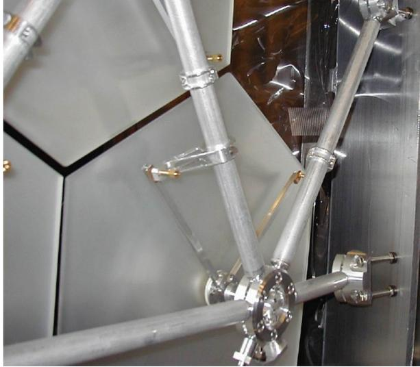
Figure 2.6: Mirror holder, which allows only angular adjustment of mirror unit around two orthogonal axes.
