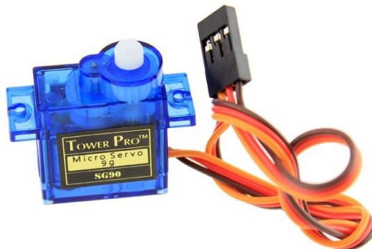
Figure 1.5: MicroServo 9g SG90. Image is from [9].
