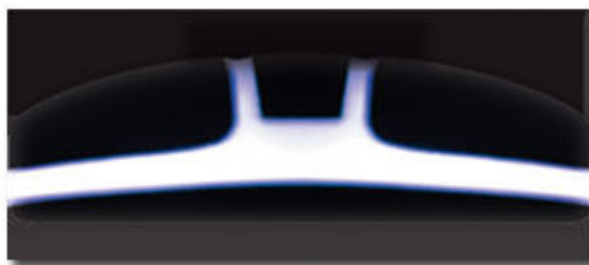
Fig. 4.1: There is uniform and homogenous plasma discharge with an atmospheric plasma surface treatment system.
