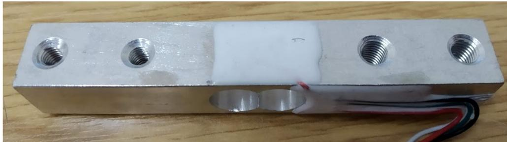
Figure 4.2: Load cell picture.
