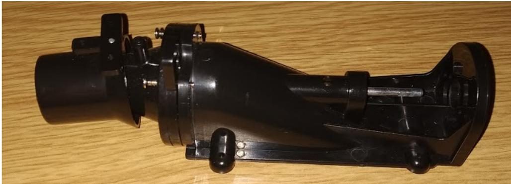
Figure 1.9: A small scale prototype of the water-jet pump to be placed inside the boat as shown at Figure 1.8.
