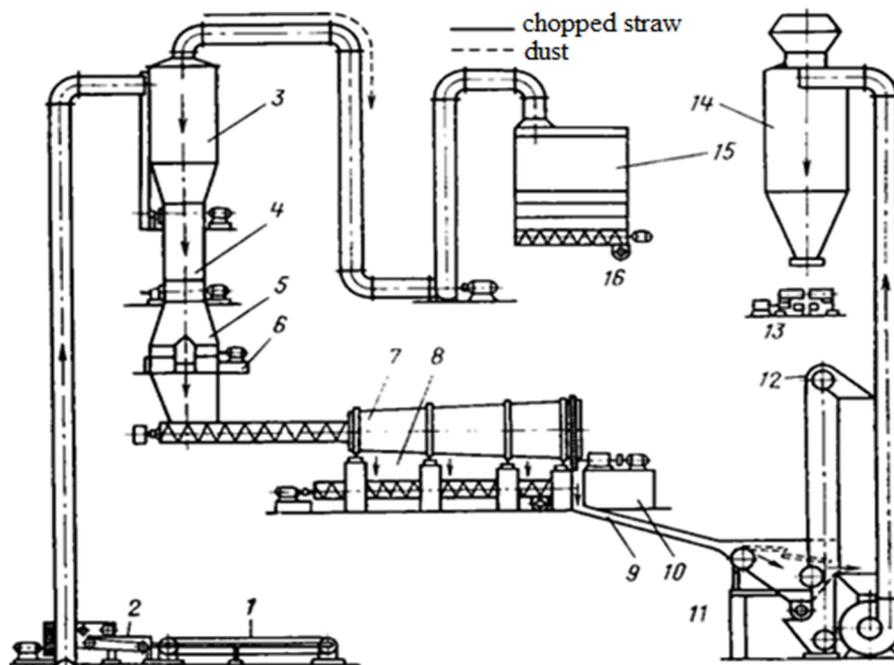
**Figure 3** Preparation and cleaning of chopped straw from straw stalks of technical hemp: 1 - untying of piles; 2 - straw chopper; 3 - preliminary dedusting; 4 - duster; 5 - shake apparatus; 6 - magnetic drum separator; 7 - vibration sorting; 8 - straw waste; 9 - conveyor; 10 - elevator; 11 - removal of grains; 12 - separation of grains; 13 - conveyor for chopped straw; 14 - cyclone; 15 - dust collection; 16 - dust removal
