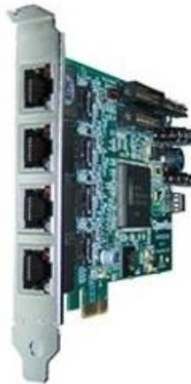
*Fig. 4: OpenVox B400E ISDN card <sup>[21]</sup>*
