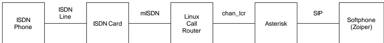
*Fig. 5: Block diagram for used setup*
