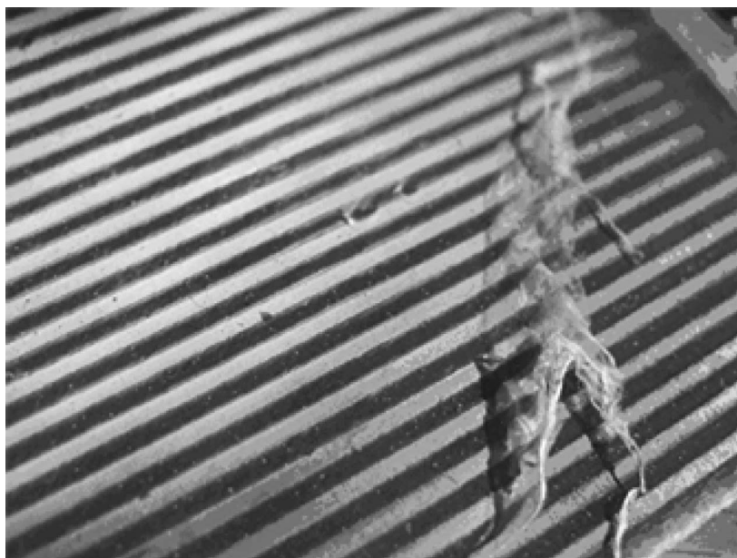
Figure 22. Special static collector consisting of Cooper strips on a laminate. Partially detached nanofibrous layer was prepared from PVA aqueous solution.
