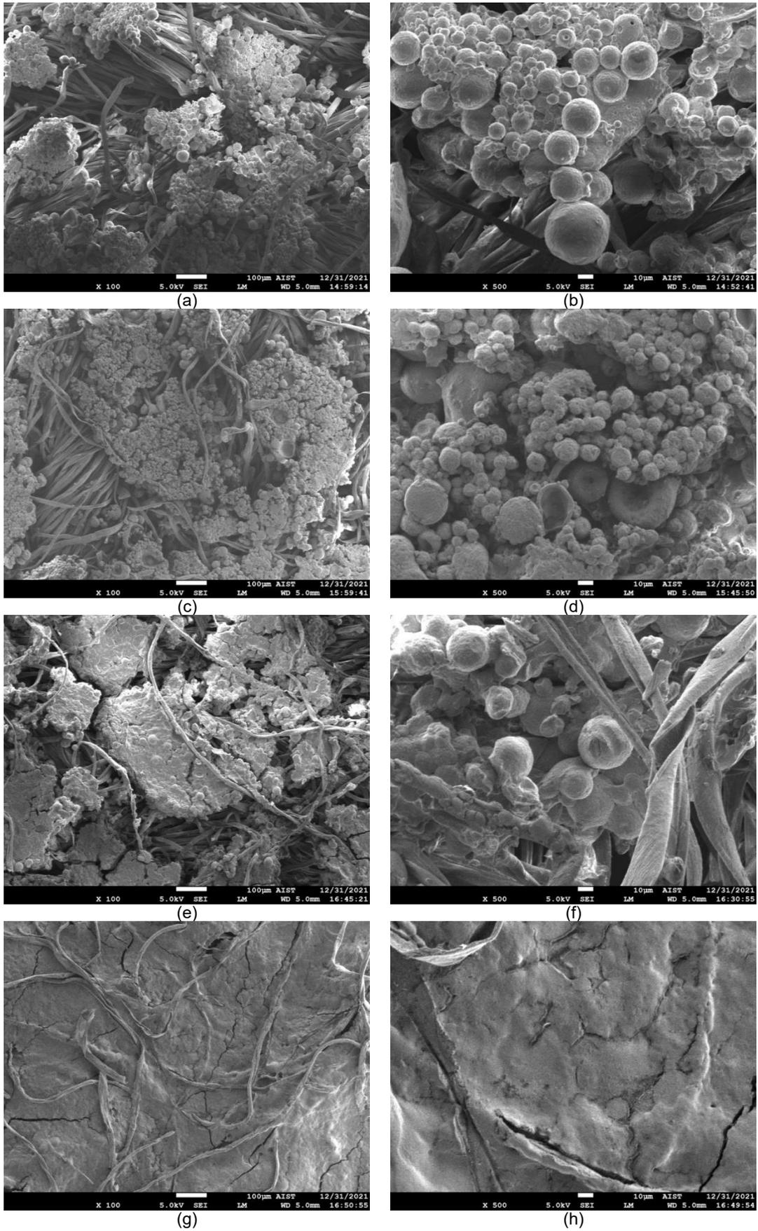
**Figure 4** SEM images of cotton interlock fabric treated with microcapsules (a,b) – treated with M1 microcapsules (0.15 g of cinnamon oil); (c,d) – treated with M2 microcapsules (0.25 g of cinnamon oil); (e,f) – treated with M3 microcapsules (0.35 g of cinnamon oil); (g,h) – treated with M4 microcapsules (0.45 g of cinnamon oil)
