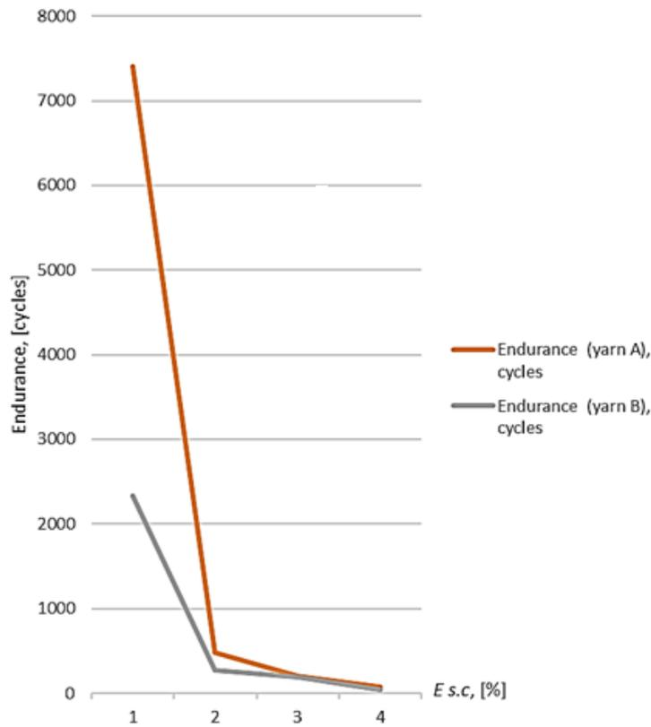
**Figure 1** Graphs of yarn endurance under repeated extensions
