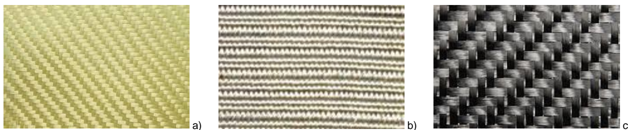
Figure 1 Industrial fabrics: a) Kevlar from para-aramid multifilament yarns 44 tex; b) Nomex from meta-aramid multifilament yarns 40 tex; c) fabric from carbon multifilament yarns 30 tex
