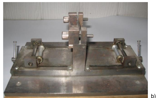
Figure 4 Scheme of the experimental unit: a) principal scheme: 1 - the yarn threading unit; 2 - metering unit for slack side tension of the yarn; 3 - metering unit for tight side tension of the yarn; 4 - unit for simulation of interaction conditions between the yarn and guides and operative parts of the textile machinery; 5 - yarn receiving unit; 6 - amplifier; 7 - analogue-to-digital converter ADC; 8 - PC; 9 - the yarn; b) central metering unit
