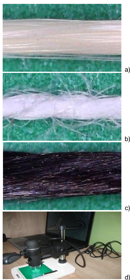
Figure 2 Yarns for experiment: a) para-aramid multifilament yarn 44 tex; b) meta-aramid multifilament yarn 40 tex; c) carbon yarn H-30 with thickness 30 tex; d) Sigeta USB digital microscope expert (magnification 10x-300x)
