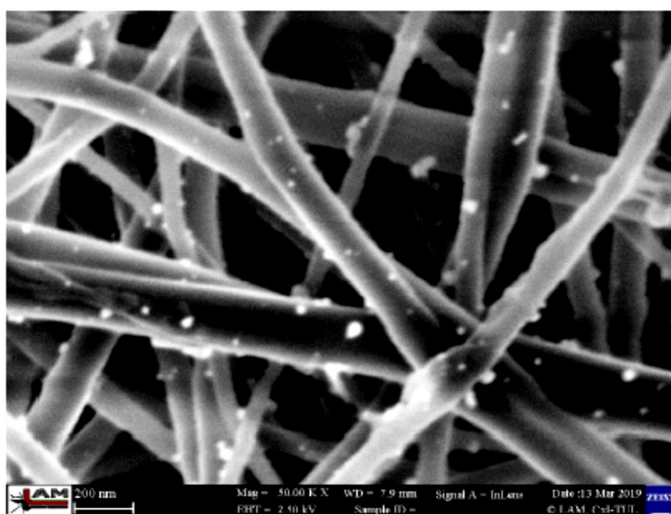
Figure S.3 FE-SEM micrograph of the Ag/PVDF-OH membrane (EHT = 2.50 kV and WD = 7.9 mm) and Mag= 50 K X, where it is possible to observe the uniform distribution of Ag NPs over the nanofibers.
