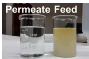
Figure 9. Feed and permeate solution for the PA6-100 nanofibrous membrane for engine oil/water separation.
