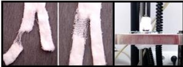
Figure 1 a) Test samples after tear strength b) Test sample during pulling through a nozzle test
