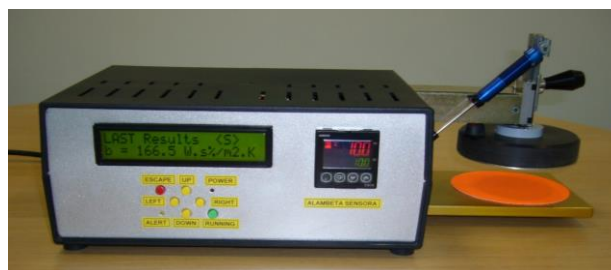
Figure 3 New ALAMBETA, a fast non-destructive tester of thermal insulation and thermal contact properties of fabrics [2]
