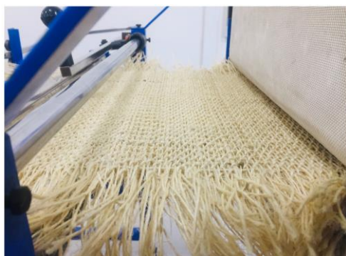
Figure 1. Development of 3D woven sisal fabric.
