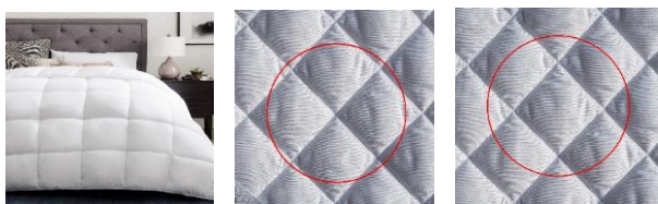
Figure 1 The appearance of a quilt blanket and a reference circular area (diameter 50 mm), determining the total seam
