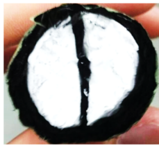
(b) Sectional view of preform
