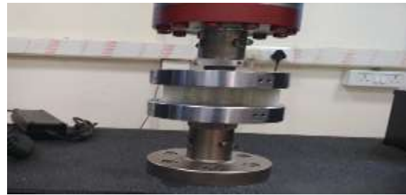
Figure.5 Flatwise compression test of Honeycomb composite
