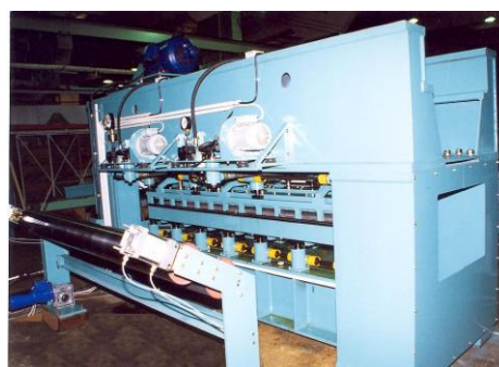
Figure 1 Needle punching machine IN-2 designed and manufactured in Research and Development Centre of Textile Machinery, Lodz, Poland
