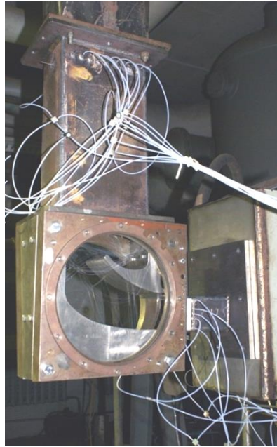
Fig. 3: Photo of sector model of diffuser (illustrative photo)
