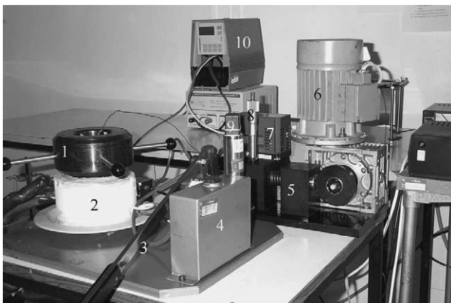
Fig. 2. Construction setup: (1) the lid of the pressure chamber with the high-pressure bushings; (2) the temperature isolation; (3) the lever of the pressure pump; (4) the oil reservoir; (5) the piston driver; (6) the engine with a transmission and a cam; (7) the speed regulator; (8) the needle valve; (9) the pressure tensometer; (10) the PID temperature regulator.
